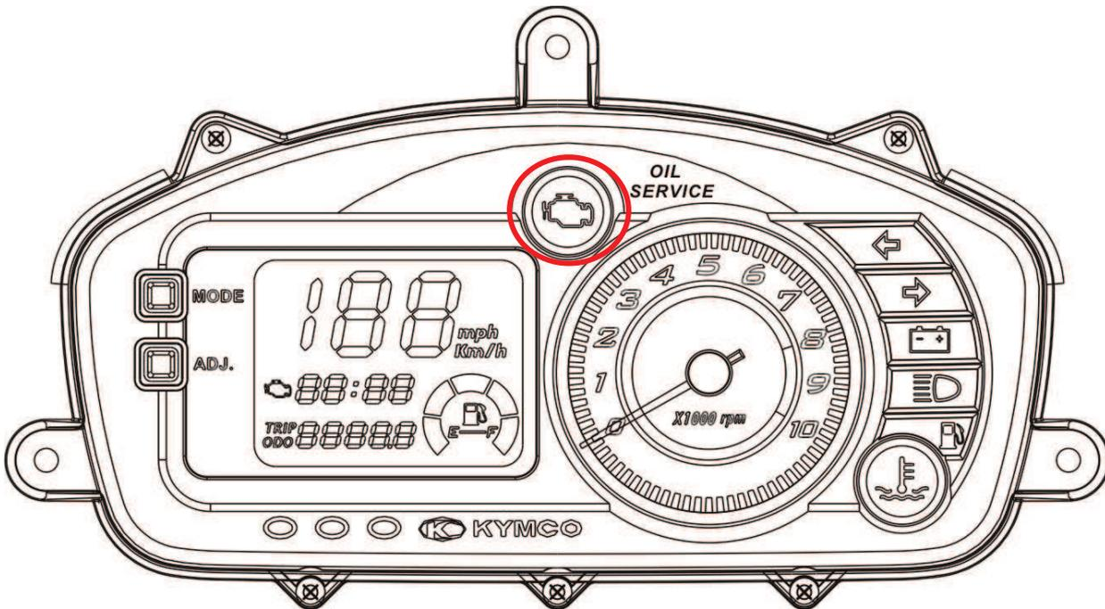
The check engine lamp (CELP) or Fi indicator is located in the center of meter.
