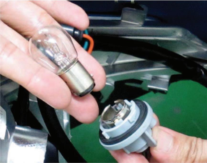
Replace the bulbs as needed. Push in and turn the bulbs counterclockwise to remove the and clockwise to install them.
