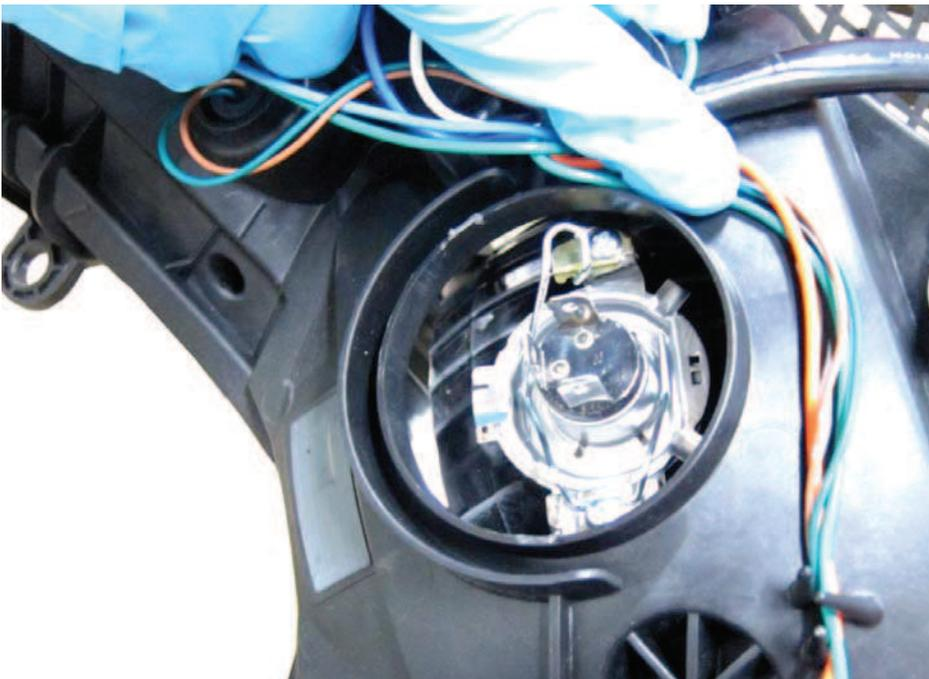
Fit the bulb into the lamp.
