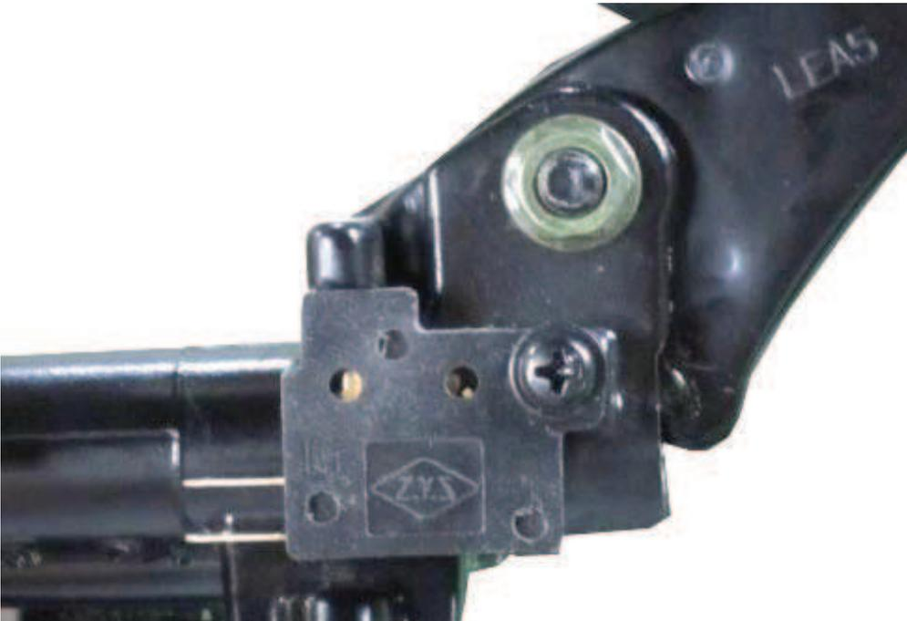
Check for continuity between the brake light switch connectors. There should be continuity when the lever is pulled and none when released.
