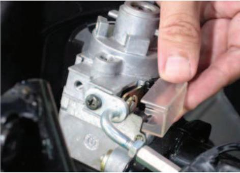
Remove the seat latch cable cover.
