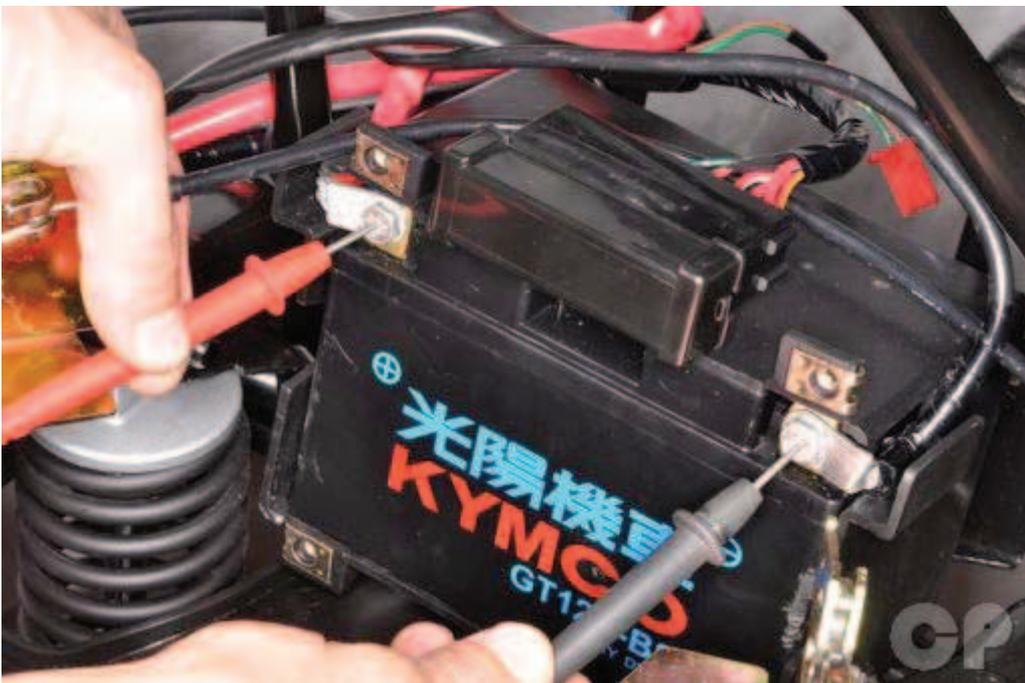
Start the engine and warm it up to the operating temperature; stop the engine. Connect the multimeter between the positive (+) and negative (-) terminals of the battery. To prevent short, make absolutely certain which are the positive (+) and negative (-) terminals or cable.
