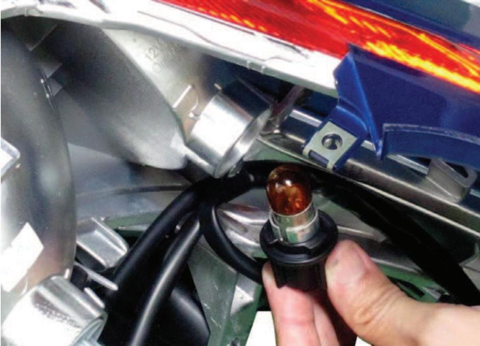
Turn the socket counterclockwise and remove it from the lamp.
