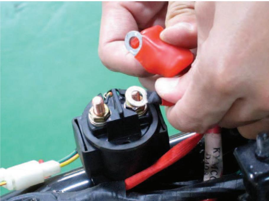
Remove the leads from the starter relay.
