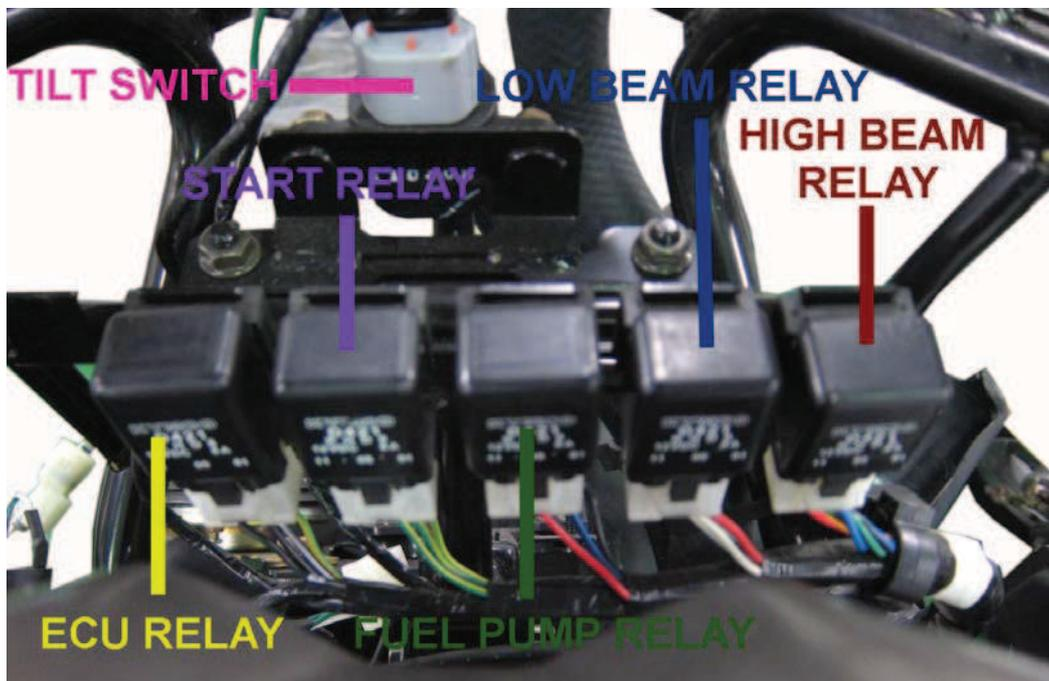
Remove and disconnect the high beam relay. The high beam relay is on the right.
