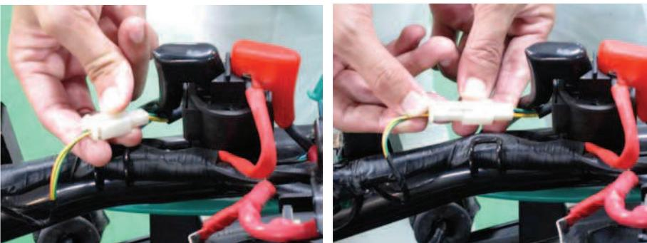
Disconnect the starter relay wire connector.
