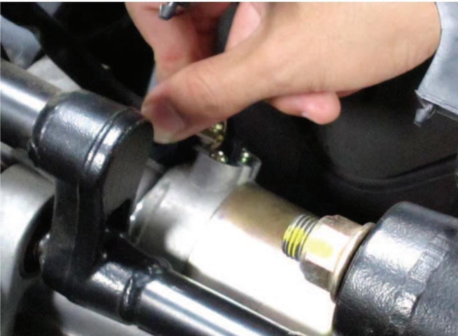
Pull back the rubber starter motor lead cover.
