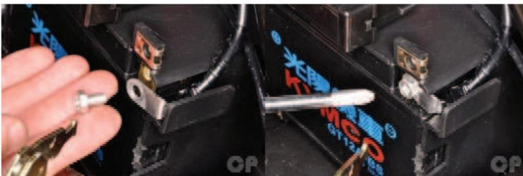
Connect the negative battery cable and install the bolt with a 10 mm socket or #3 Phillips screwdriver.
