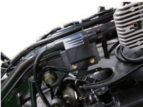
Remove the two ignition coil mounting bolts with an 8 mm socket.
