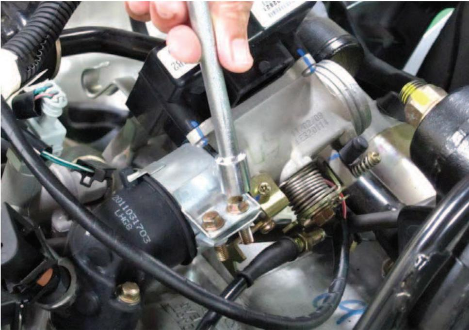
Loose two nuts attaching to the holder intake pipe.
