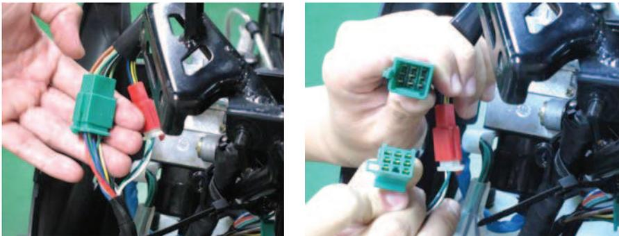
Unplug the green connector for the right handlebar switches.
