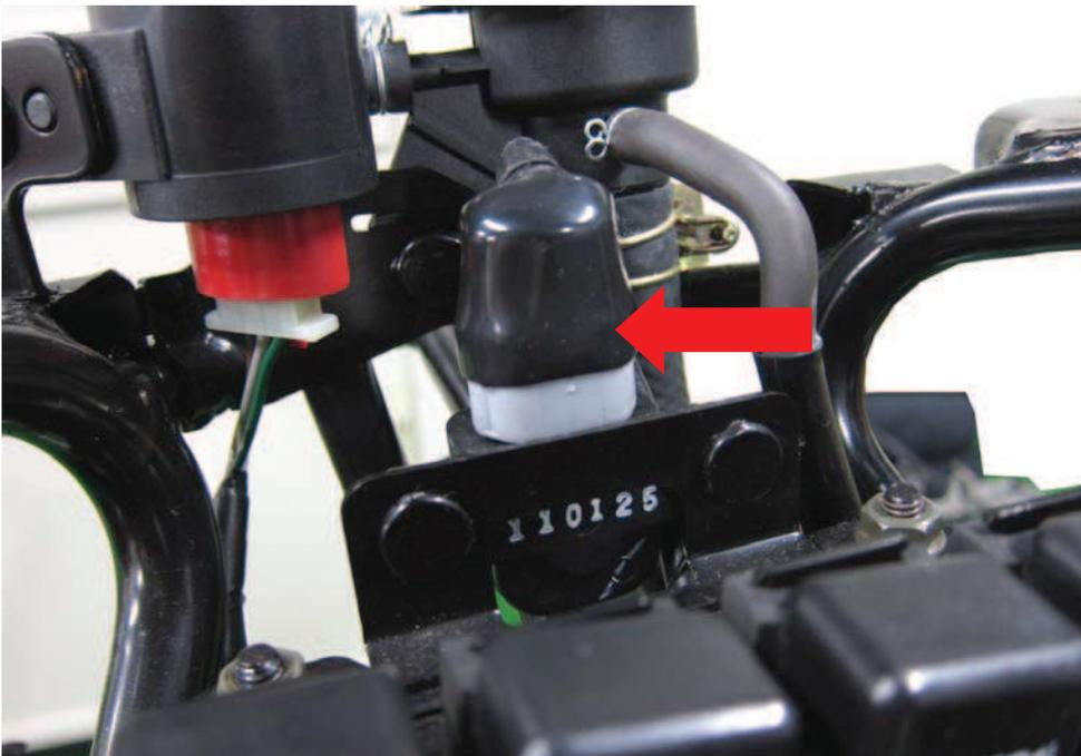
The tilt switch is located in the front near the radiator cap.
