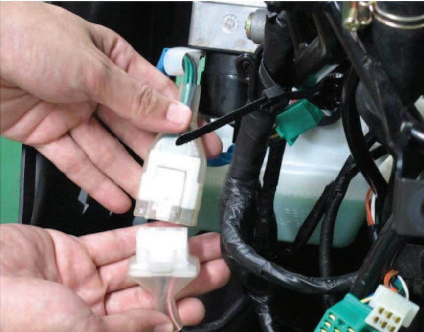
Unplug the white six-pin ignition switch connector.
