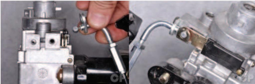
Fit the end of the seat latch cable into the ignition switch.
