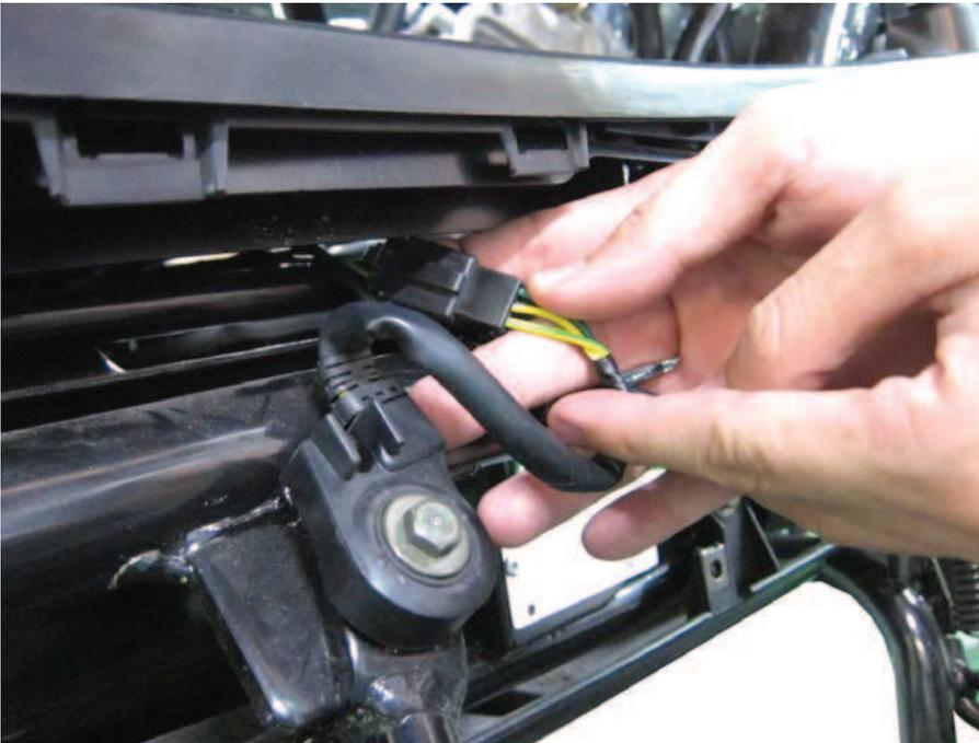
Unplug the three-pin side stand switch connector.
