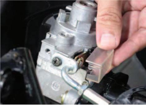
Install the seat latch cable cover.
