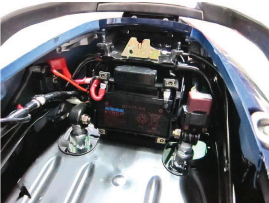
The fuse box is located on top of the battery.
