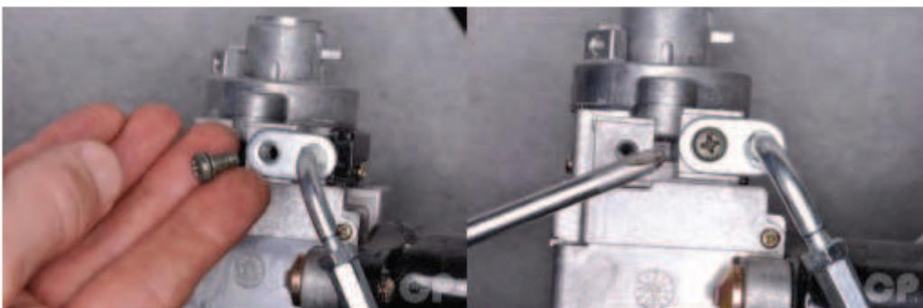
Install the seat latch cable screw and tighten it securely with a #2 Phillips screwdriver.
