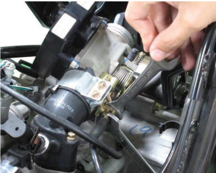
Loose two nuts attaching to throttle cable with 10mm&12mm sockets, and then remove the throttle cable.
