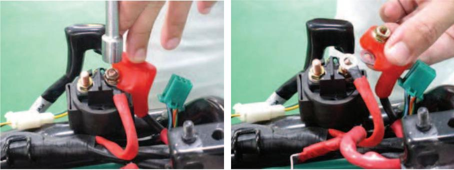
Remove the nuts that hold the starter motor lead and battery lead wires to the starter relay with a 10 mm socket.
