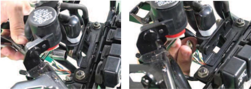
Remove the two tilt switch nuts with a 10mm socket.
