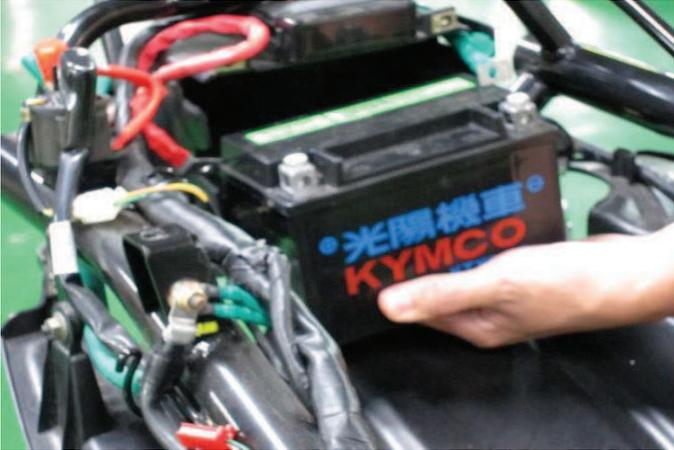
Fit the battery into the battery tray.
