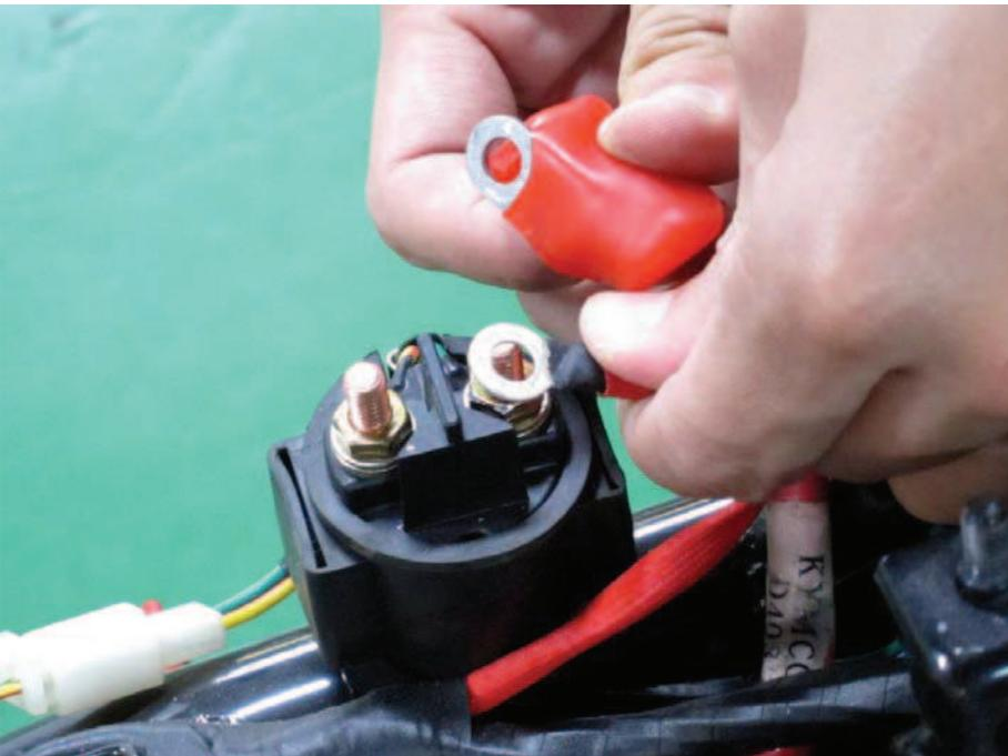
Remove the leads from the starter relay.
