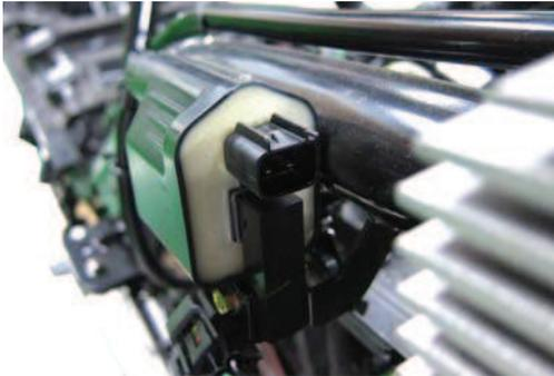
Remove the ignition coil leads.
