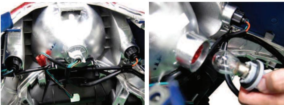
Remove the taillight socket with bulb from the tail light housing by turning it counterclockwise.
