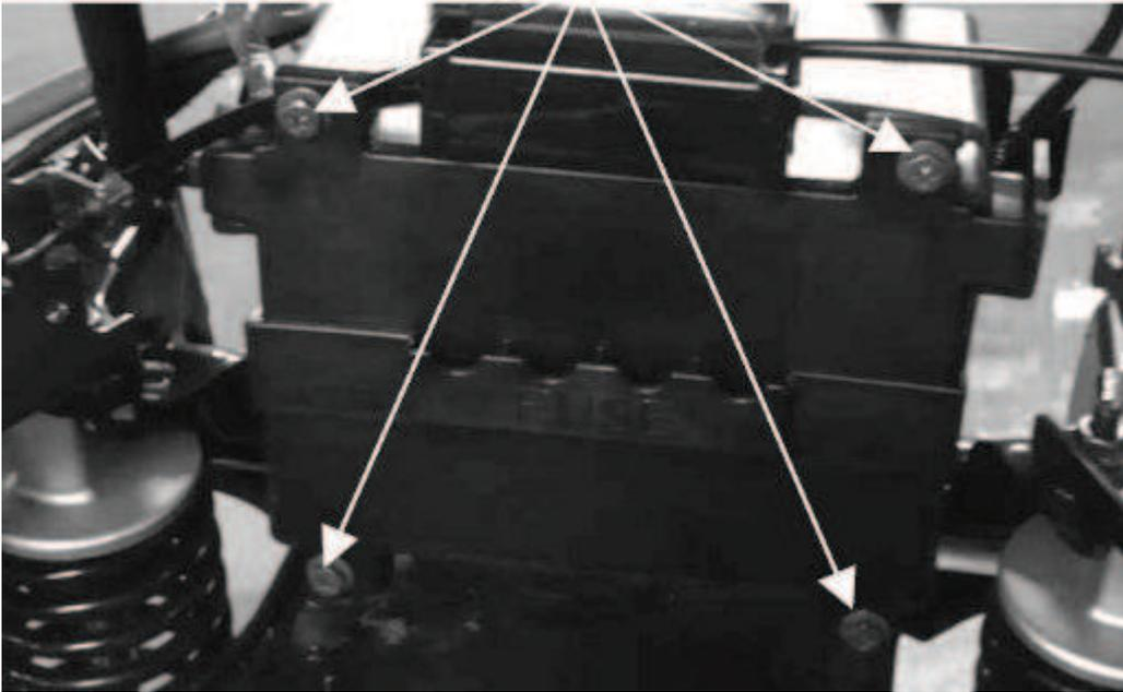
Install the battery cover. Install the four battery cover screws and tighten them securely.
