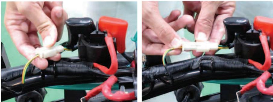
Disconnect the starter relay wire connector.
