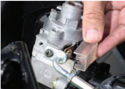
Remove the seat latch cable cover.
