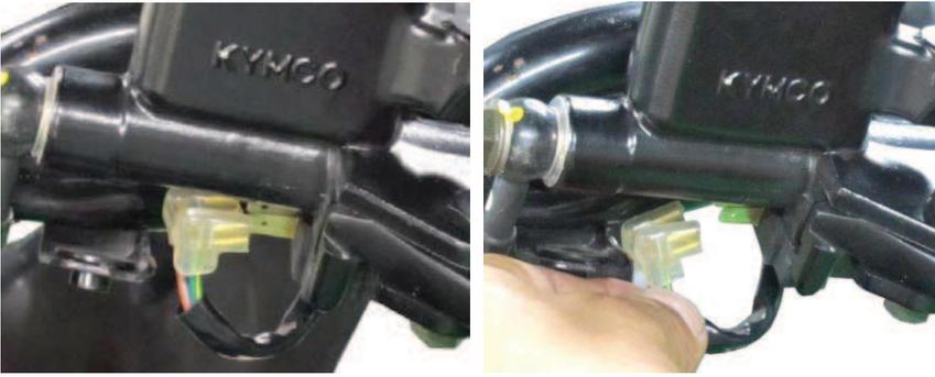
Unplug the brake light switch connectors.
