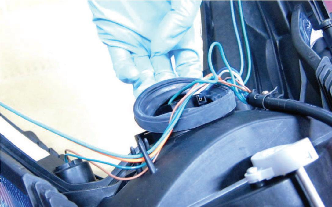
Fit the rubber cover into place. Make sure the rubber covers are secured in place.
