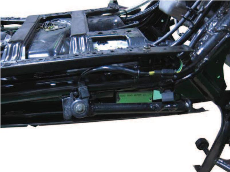
With the side stand retracted there should be continuity between the yellow/green wire and the green wire terminals.
