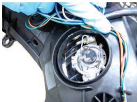
Slide back the rubber headlight covers. Remove the clip with a screwdriver.
