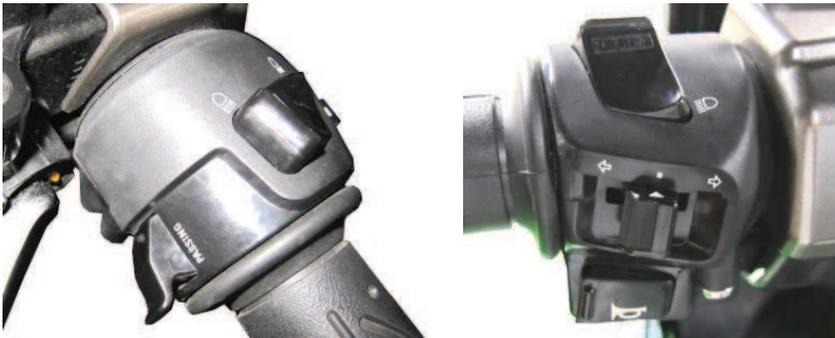
Use a digital multimeter to check for continuity to inspect the handlebar switches. Continuity should exist between the wires as indicated.
