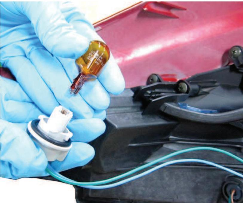
Push in on the bulb and rotate it clockwise to remove it from the socket. Insert the new bulb. Push down on the bulb and rotate it counterclockwise to lock it into place.
