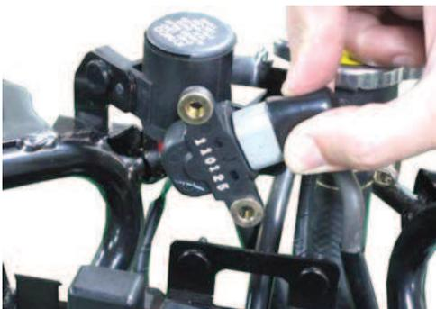
Incline the tilt switch  $65 \pm 10$  degrees to the left or right at the ignition switch "ON". Measure the voltage as below.
