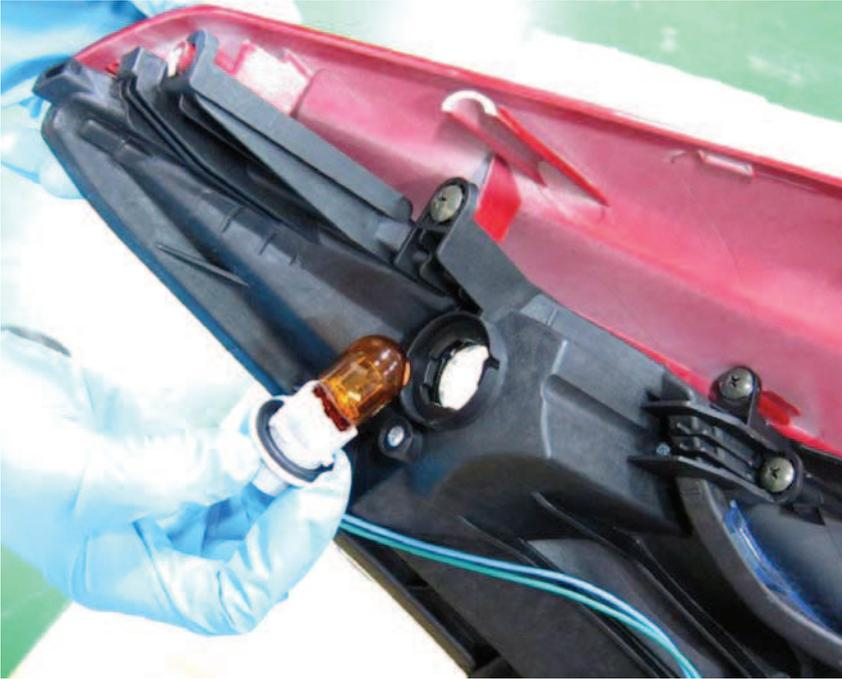
Insert the turn signal bulb and socket into place. Turn the socket clockwise to lock it into place.
