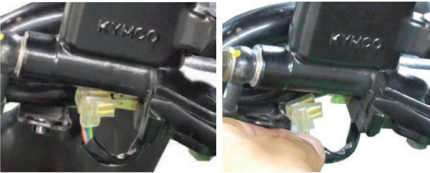
Unplug the brake light switch connectors.
