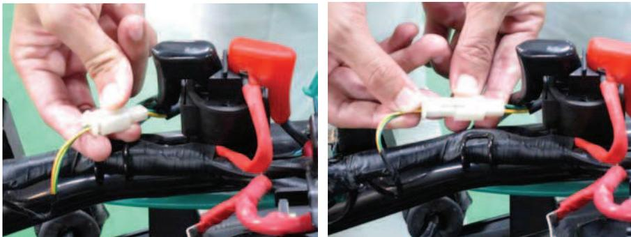
Disconnect the starter relay wire connector.
