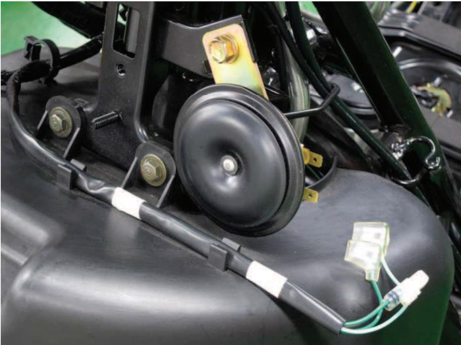
Disconnect the horn connectors from the horn. Connect a 12 V battery to the horn terminals. The horn is normal if it sounds when the 12 V battery is connected across the horn terminals.
