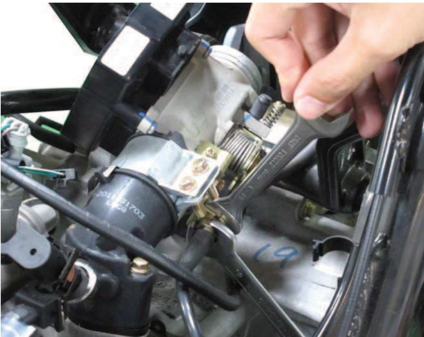
Loose two nuts attaching to throttle cable with 10mm&12mm sockets, and then remove the throttle cable.
