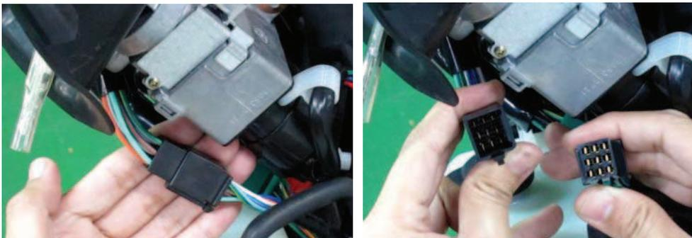
Unplug the black connector for the left handlebar switches.
