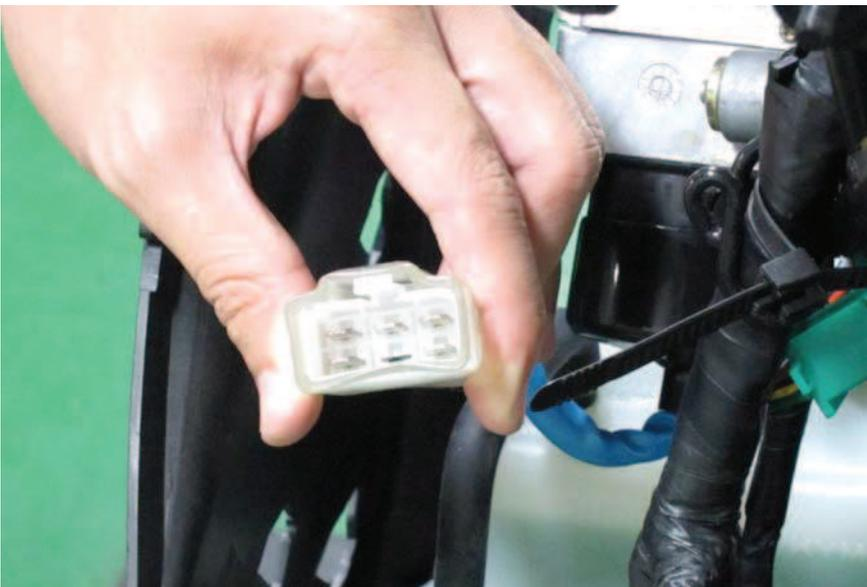
Use a digital multimeter to check for continuity to inspect the ignition switches. Continuity should exist between the wires as indicated.
