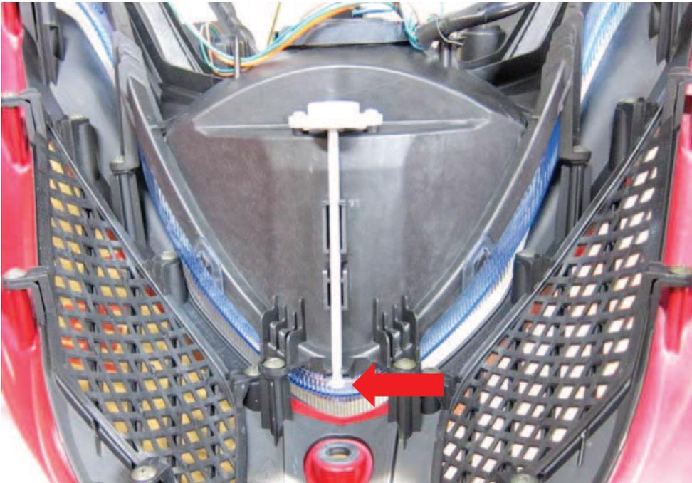
Turn the screws to adjust the head light aim as needed.
