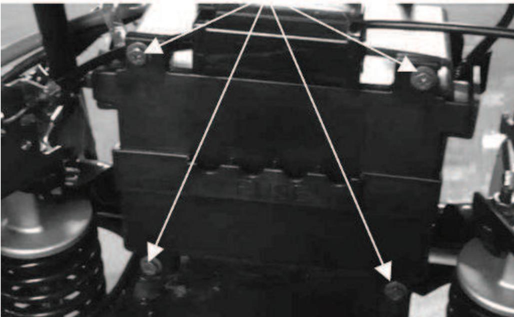
Remove the four battery cover screws. Remove the battery cover.
