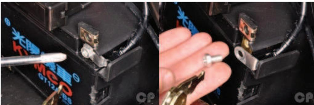
Remove the negative battery cable bolt with a 10 mm socket or #3 Phillips screwdriver. Free the negative cable from the battery.
