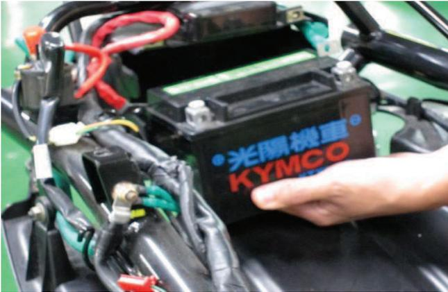
Lift the battery out of the battery tray.
