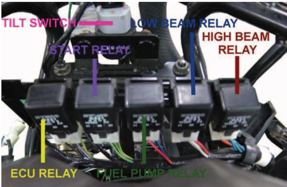
The fuel pump relay is located in the front under the dash panel. Remove and disconnect the fuel pump relay.
