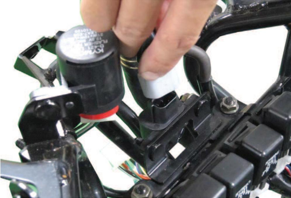
Disconnect the connector to remove the tilt switch.
