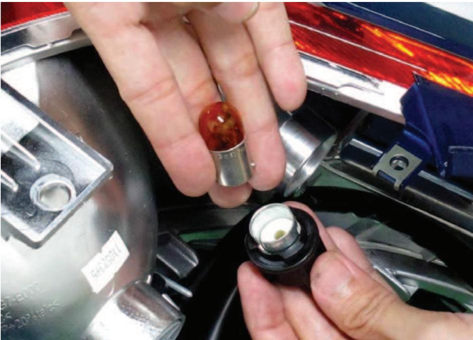
Push in the bulb and turn it counterclockwise. Remove the bulb. Insert the new bulb and turn it clockwise to lock it in place.
