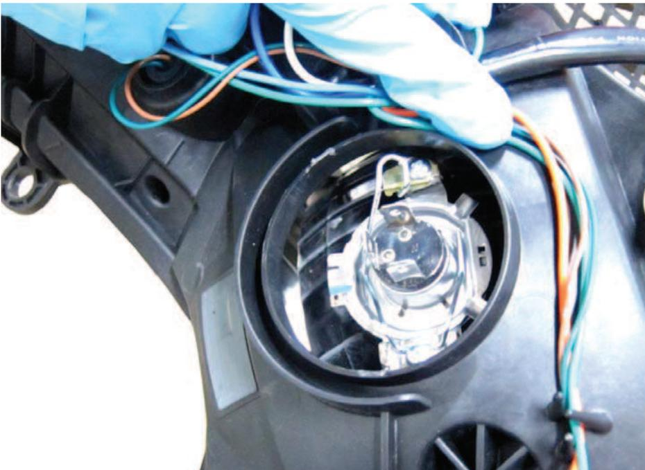
Fit the bulb into the lamp.
