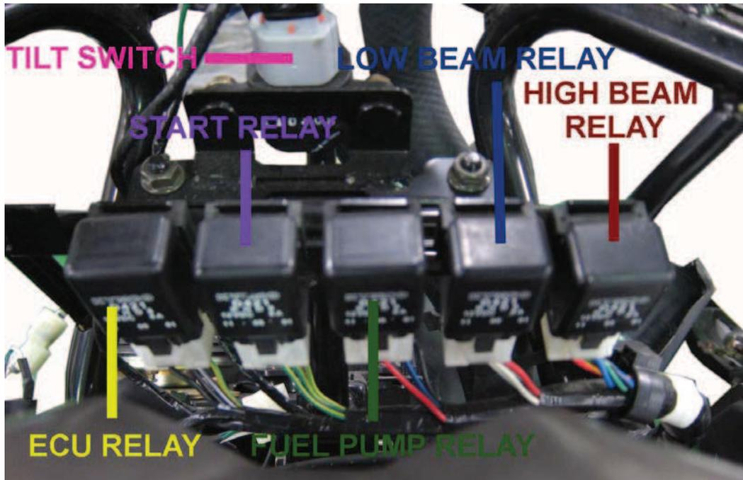
The ECU relay is located in the front under the dash panel, to the left of the start relay. Remove and disconnect the ECU relay. Disconnect the dash if needed. See the [Dash](#) topic for more information.
