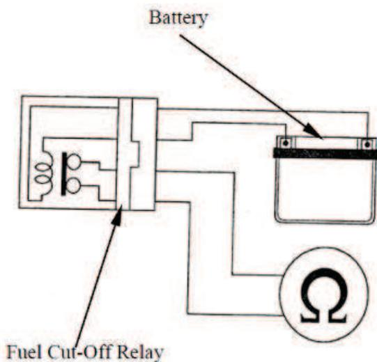
Connect the multimeter to the fuel cut-off relay connector terminals.
