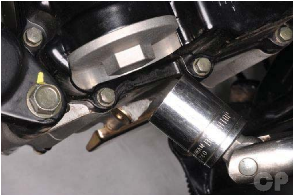
Loosen the oil filter cap with a 24 mm socket.
