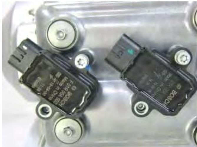
Clean off the area surrounding the spark plug with compressed air or a shop towel to make sure debris doesn't get into the combustion chamber when the spark plug is removed.
