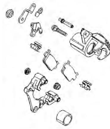
Loosen and remove the two bolts of rear caliper. The bolts are with blue Loctite (non-permanent) to the threads. Using this type of bolts when installation. Installation torque: 3~4 kgf-m (30~40 N-m)
