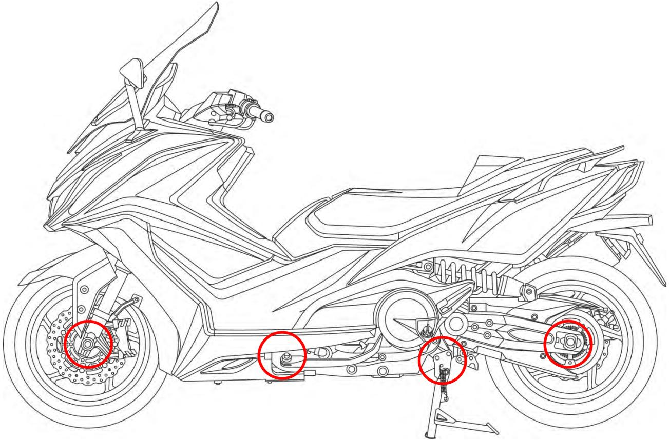
The frame lubrication points are listed below. Use general purpose grease. Apply clean engine oil or grease to cables and movable parts not specified. This will avoid abnormal noise and increase the durability of the motorcycle.
