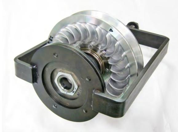
Secure the spring compressor tool in a vise. Loosen the plate nut with the socket. And remove the plate nut of driven pulley set.
