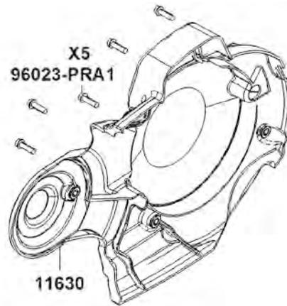
Remove two bolts and remove the CVT cover element.
