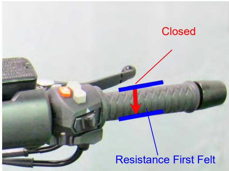
Check the throttle cable free play by gently rotating the throttle grip back until resistance is felt.
