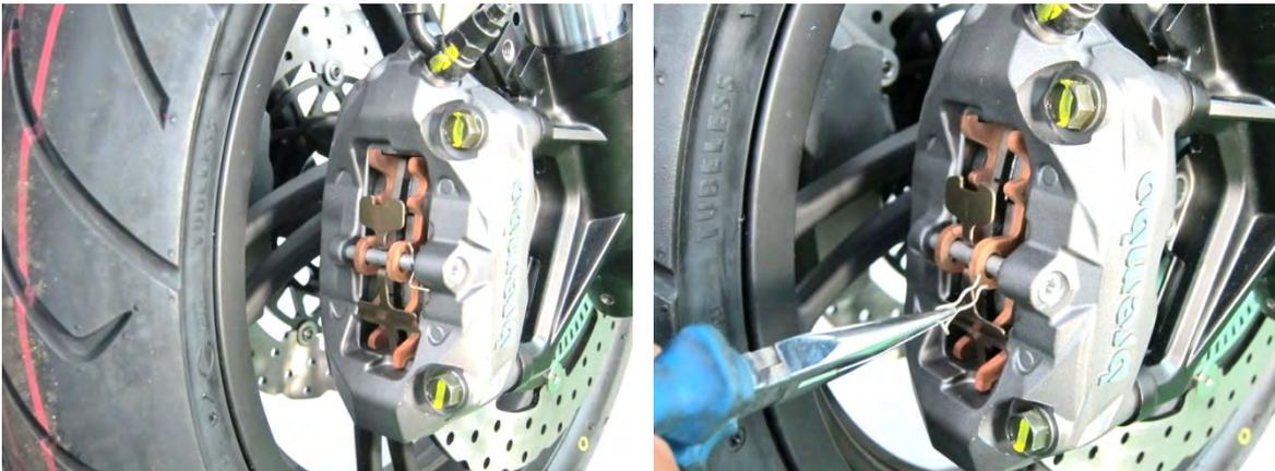
Remove the screw, loosen the brake pad.
