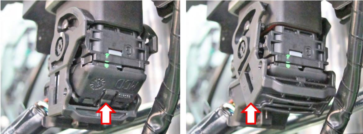
Remove the nuts and bracket to remove the ECU.
