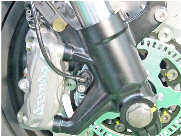
Inspect the wheel speed sensors, rotors, wires, and connectors if the speed doesn't show correctly.
