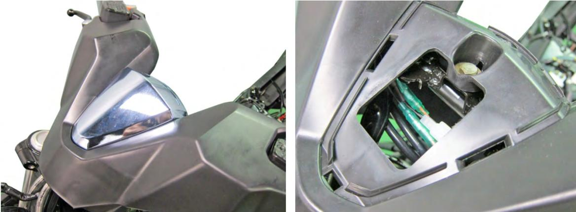
Remove the bolts, screws.
