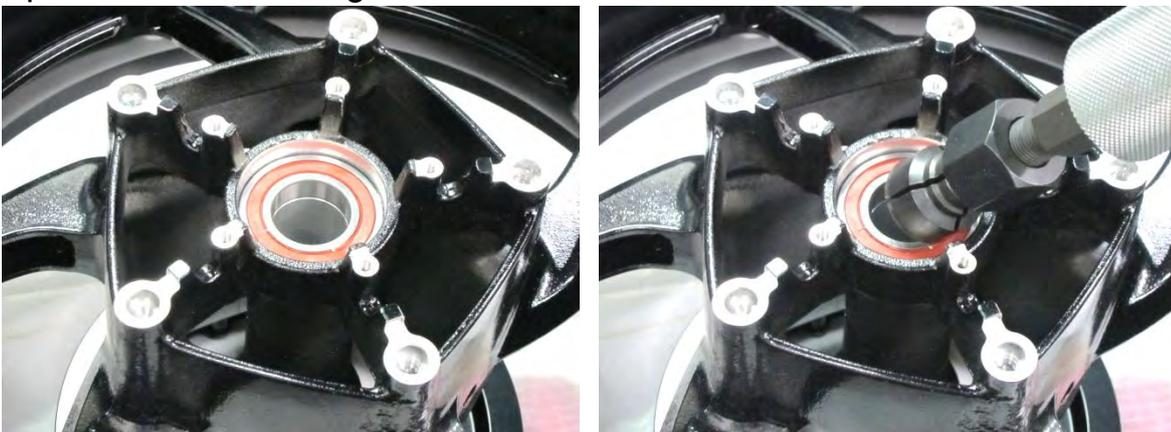
Heat the bearing area of the wheel with a heat gun, take the bearing out of the freezer and install it. You can use a bearing installer tool or a socket with the same outside diameter as the bearing. Make sure the bearing is fully seated and the marked side is facing out.
