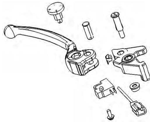
Check for continuity between the brake light switch connectors. There should be continuity when the lever is pulled and none when released.
