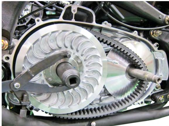
Lubricate the threads of the nut before installation.
