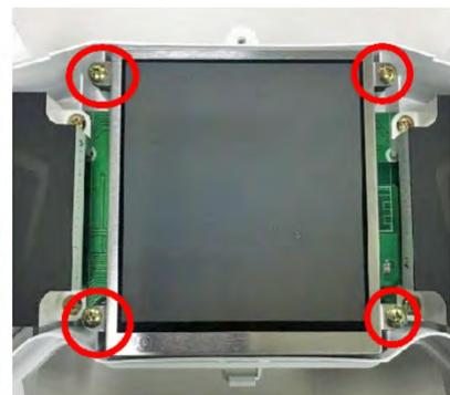
Remove the TFT module and replace with a new one.
