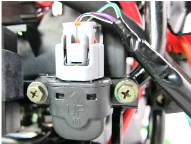
Place the tilt switch vertical as shown and the ignition switch "ON". Measure the voltage as below.
