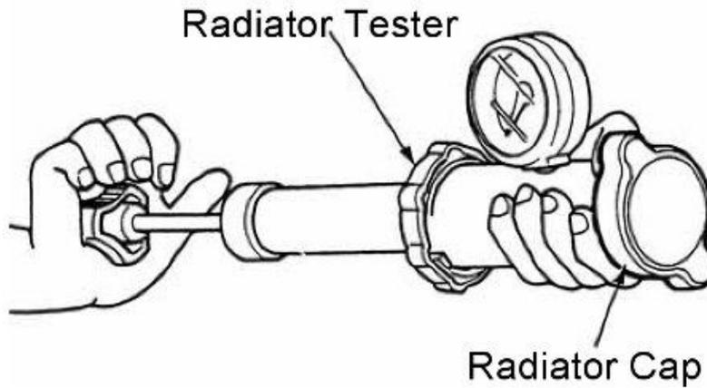
Wet the seal on the radiator cap and install it to the pressure tester. Replace the cap if it does not relieve the pressure as specified.
