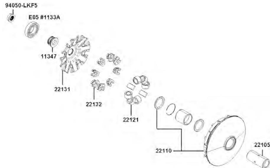
Inspect the faces of the drive pulley. Clean away any grease from the faces.
