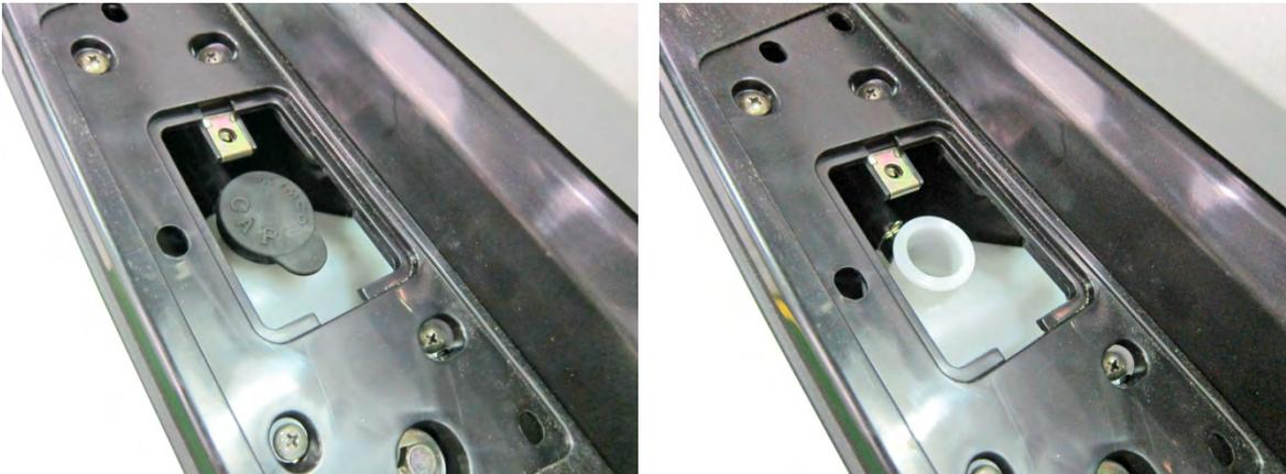
Open the coolant reserve tank lid. Siphon the coolant out of the reserve tank with an appropriate suction device. If a suction device is unavailable remove the reserve tank and pour it out.
