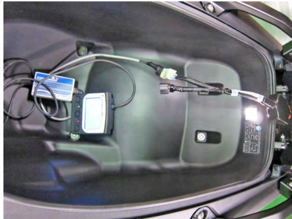
OBD diagnostics connector (part number:36205-LGC6-E00) and can linker .
