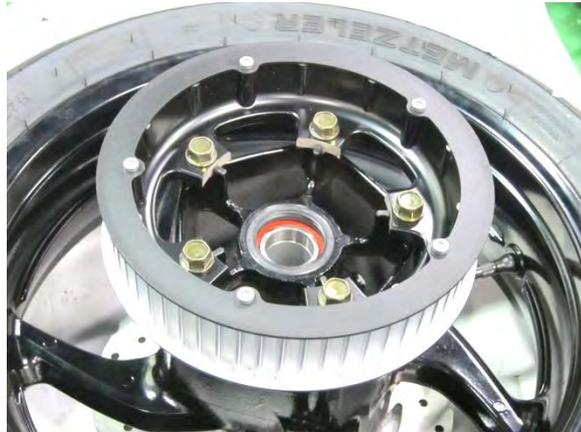
Remove the five bolts of the driven belt sprocket.
