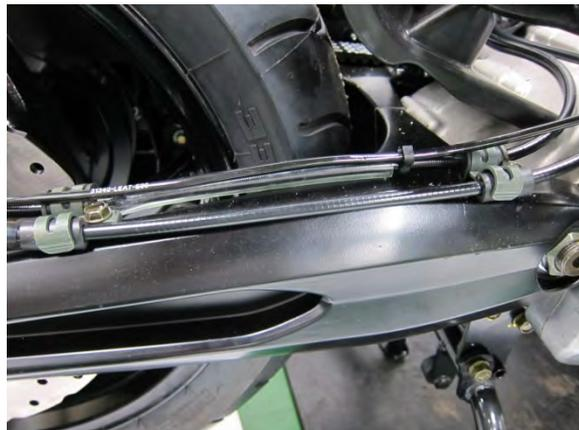
Remove the bolt of rear fixed plate.
