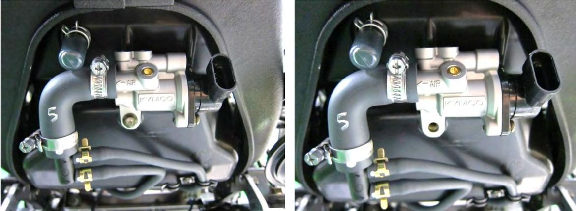
Remove the ISC screw with a #2 Phillips.
