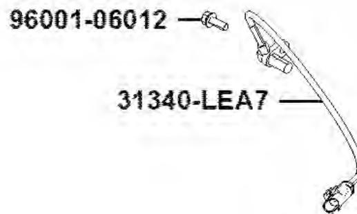
Release the cable of speed sensor.
