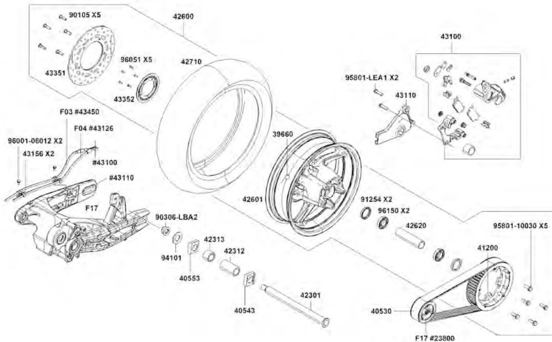
Loosen the fixed nut (front), rotate the adjust bolt (rear) counter clockwise and move wheel forward to loosen the belt.
