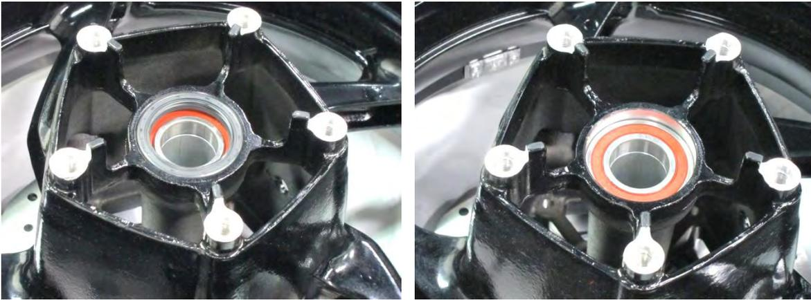
Replace the bearings if the races do not turn smoothly, quietly, or if they fit loosely in the hub.
