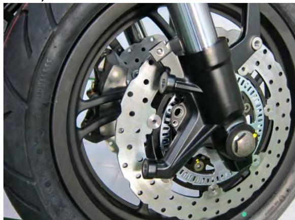
Remove the bolt of front axle.
