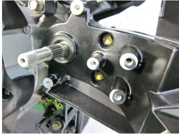
Remove the two bolts and nuts of left rear fork. And Slide out and remove the left rear fork.
