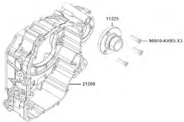
The bolts are all with blue Loctite (non-permanent) to the threads. Using this type of bolts when installation.
