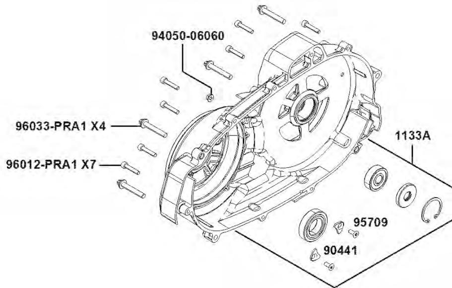
Inspect the belt case bearing by turning it with a finger. Replace the bearing if it is rough or noisy.
