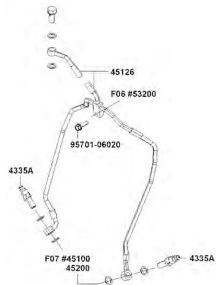
Replace the brake hose banjo bolt sealing washers with new items on assembly.
