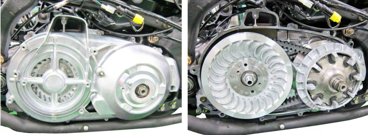
Remove the gasket and two dowel pins.
