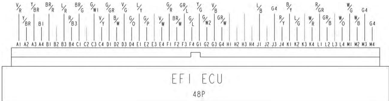
Check for continuity between pin M3 and M4 of the ECU side connector.
