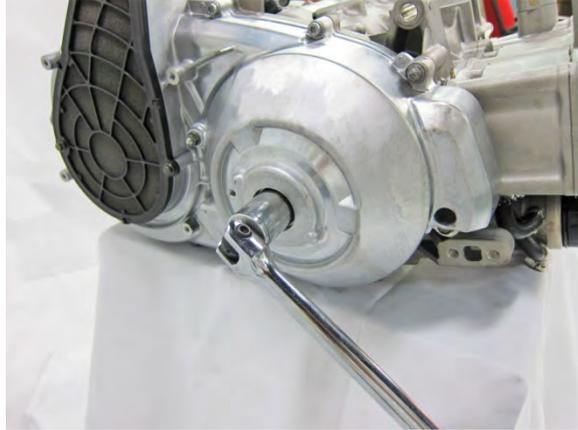
Rotate the crankshaft to TDC mark.
