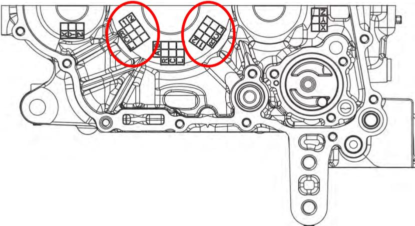
Balancer gear shaft and crankcase plane bearing color selection follows the below charts.
