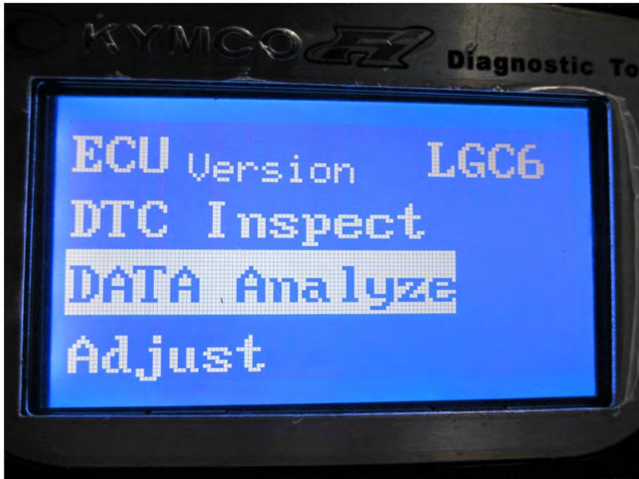
Press the down button (right) to move the item selector down to the DATA Analyze item. Press enter to bring up the DATA Analyze page 01 shown below. Press the down button to continue through the seven DATA Analyze pages.
