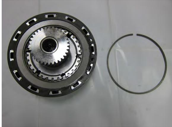
Remove the retainer and spring.
