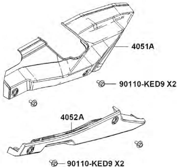
Loosen and remove the three bolts.
