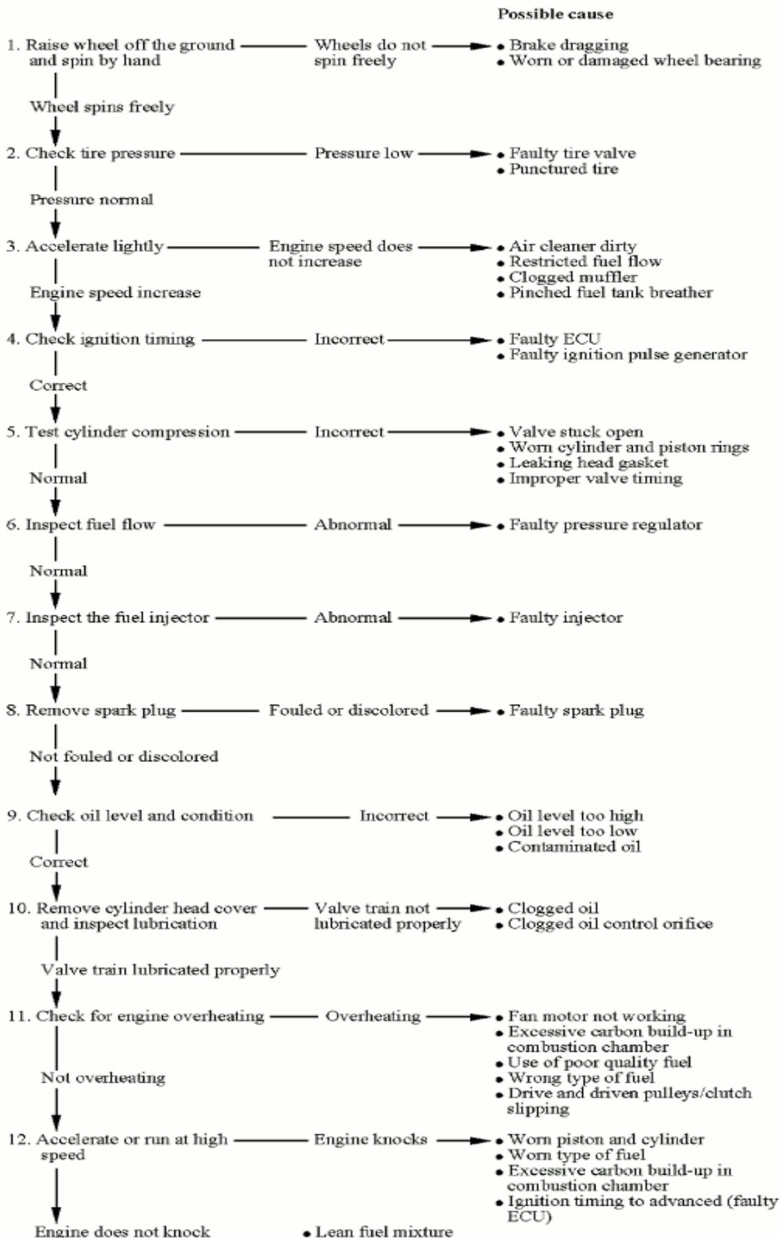
**POOR PERFORMANCE AT LOW AND IDLE SPEED**
