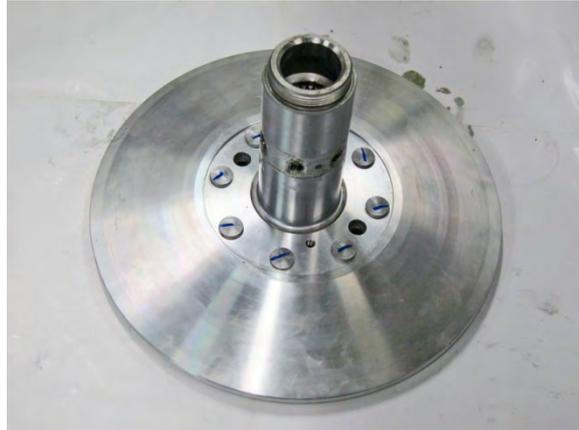
Replace the seals from the driven pulley.
