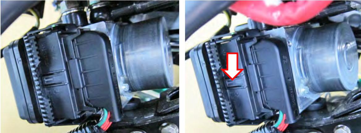
Press the claw to release the coupler of ABS module.
