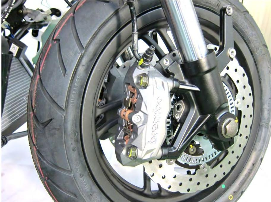
Remove the snap clip of the pin.
