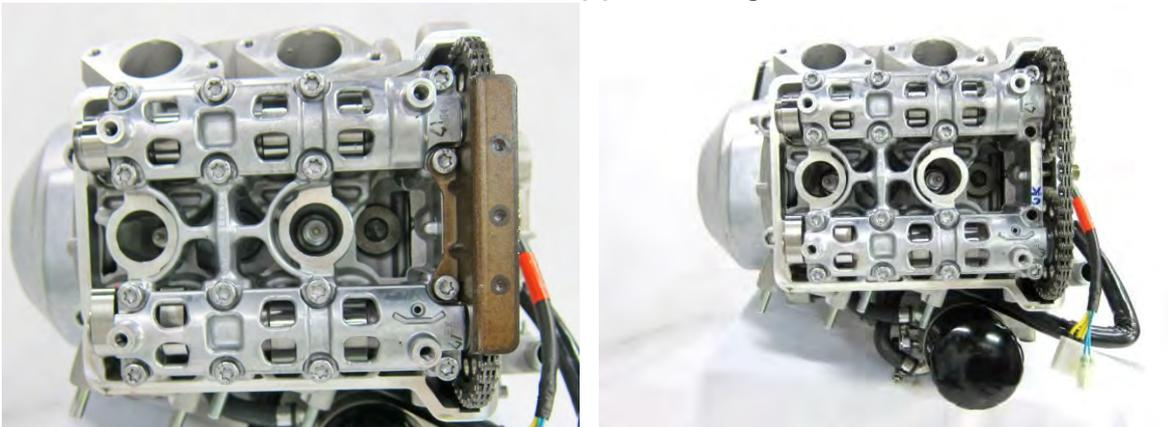
Loosen and remove the camshaft holder bolts in a crisscross pattern in several steps, then remove the camshaft holder. And remove camshafts.
