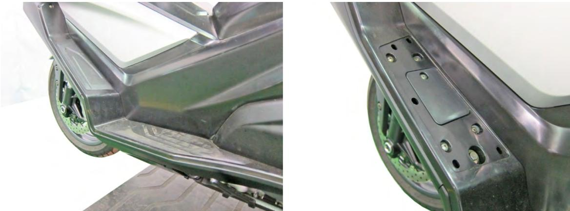
Remove the engine coolant lid screw, and remove the engine coolant lid.
