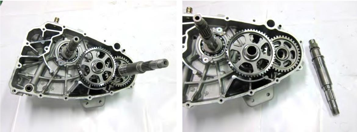
Remove the counter A gear and remove the final gear.
