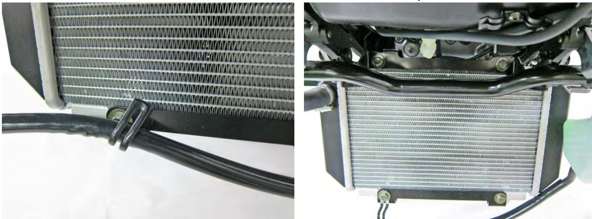
Remove the radiator from the frame.
