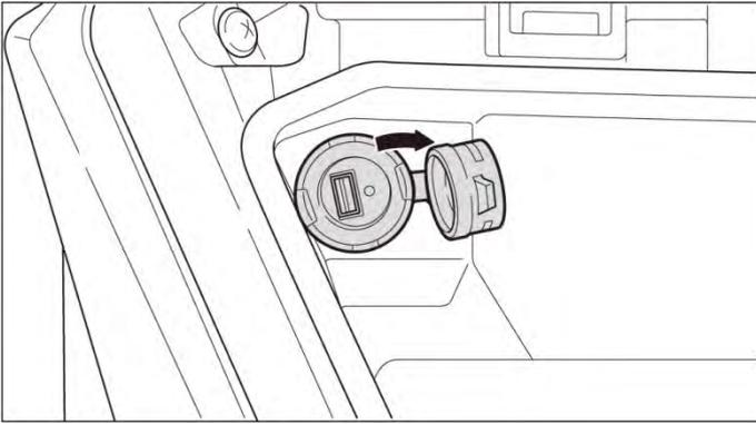
This vehicle is provided with a USB Power Socket. You may connect a low power consumption product to the Socket, for charging the product while the engine is running.
