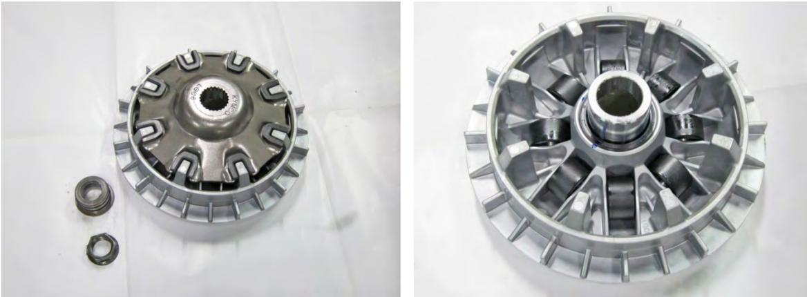
Remove the rubber damper pieces from the ramp.
