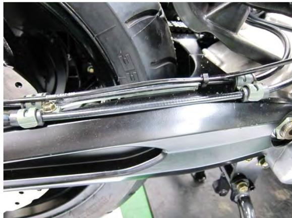
Remove the bolt of rear fixed plate.
