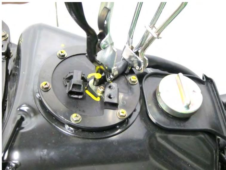
Remove the fuel pump mounting bolts.
