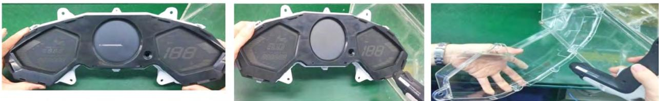
Install the cover of meter firmly and install the screws crisscross evenly.
