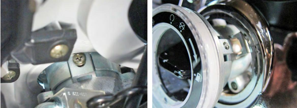
Remove the screws, remove the seat and fuel cap latch cables from the ignition switch.
