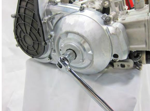
Rotate the crankshaft to TDC mark.
