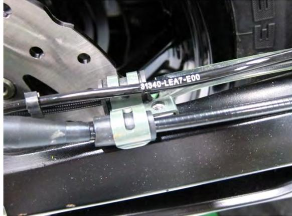
Remove the bolt of front fixed plate.
