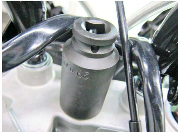
Remove the washer of bottom bridge.
