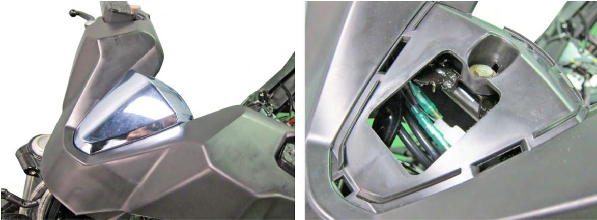
Remove the bolts, screws and remove the handle bar heater connectors.
