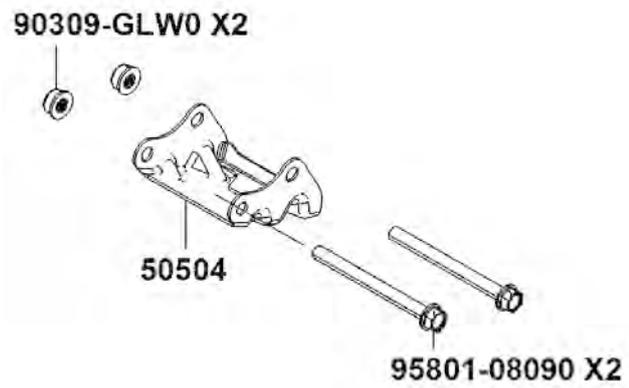
Remove the bolt, nut and upper plate.
