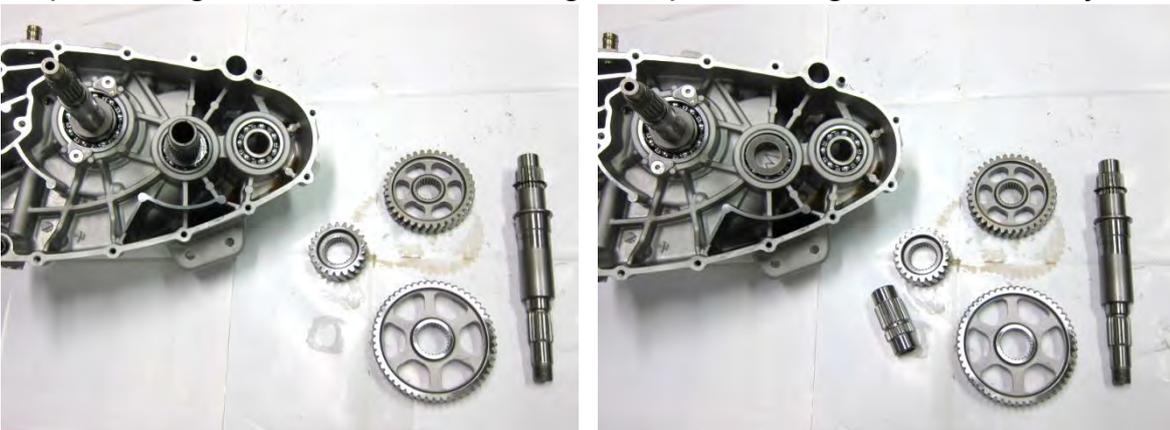
Remove the washer and remove the drive shaft.
