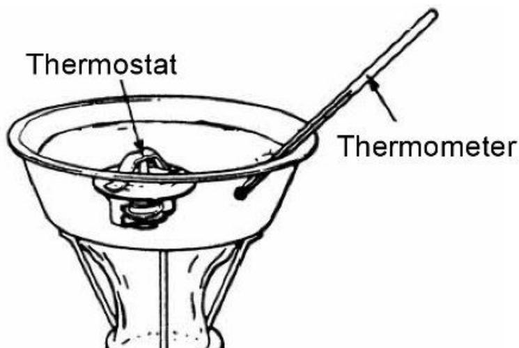
Suspend the thermostat and a thermometer in a pot of water with string. Make sure the thermostat and the thermometer are not touching the pot. Bring the temperature up to the specification slowly and check the operation of the thermostat.
