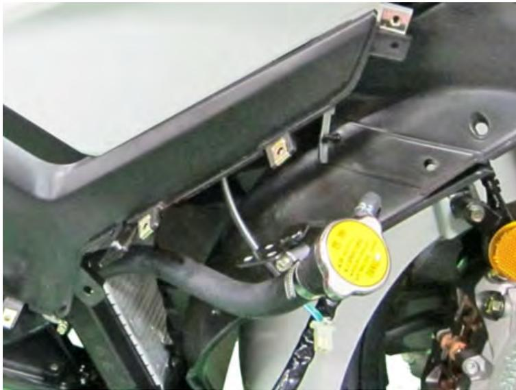
Remove the radiator cap in two stages. Allow any built up pressure to vent and then open the cap all the way and remove it.
