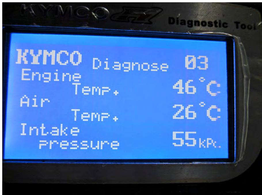
The 03 page shows engine temperature, air temperature, and intake pressure.
