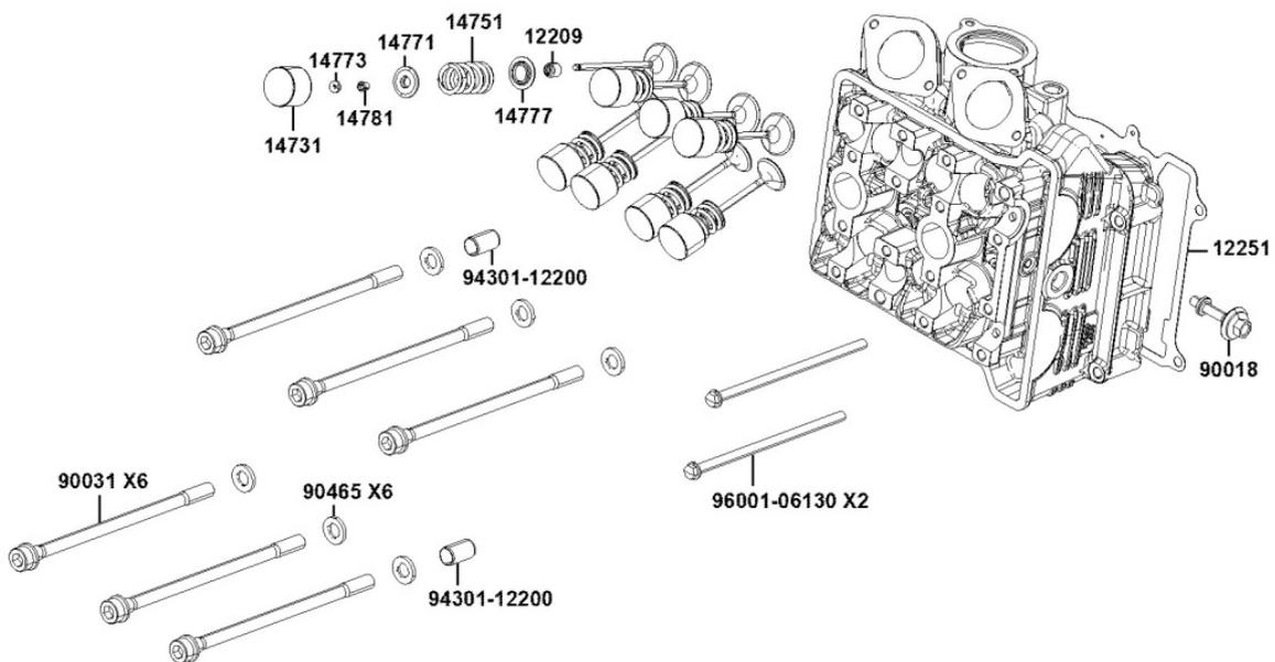
Installation: The bolts mounting order and torque at 3 stages follow the below rule.
