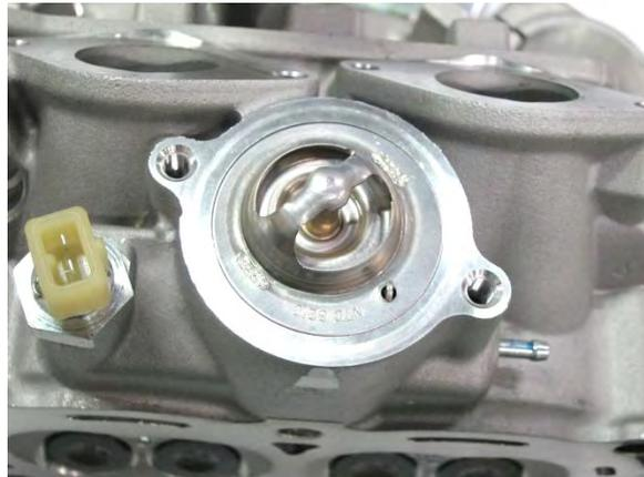
Lift out and remove the thermostat.
