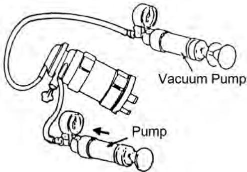
NOTE: Always using the pump by manual, do not apply high pressure for testing to prevent the valve from malfunction.
