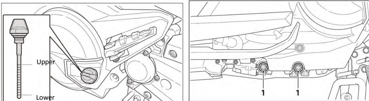
2. Clean Oil Filter and re-install it. Tighten Drain Cock after wiping it clean.
