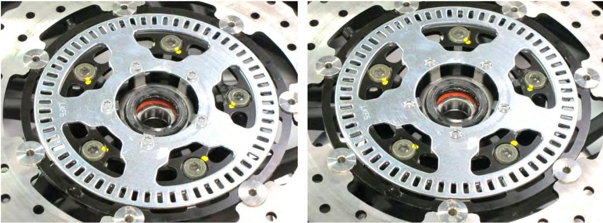
Remove the bolts of brake disk.
