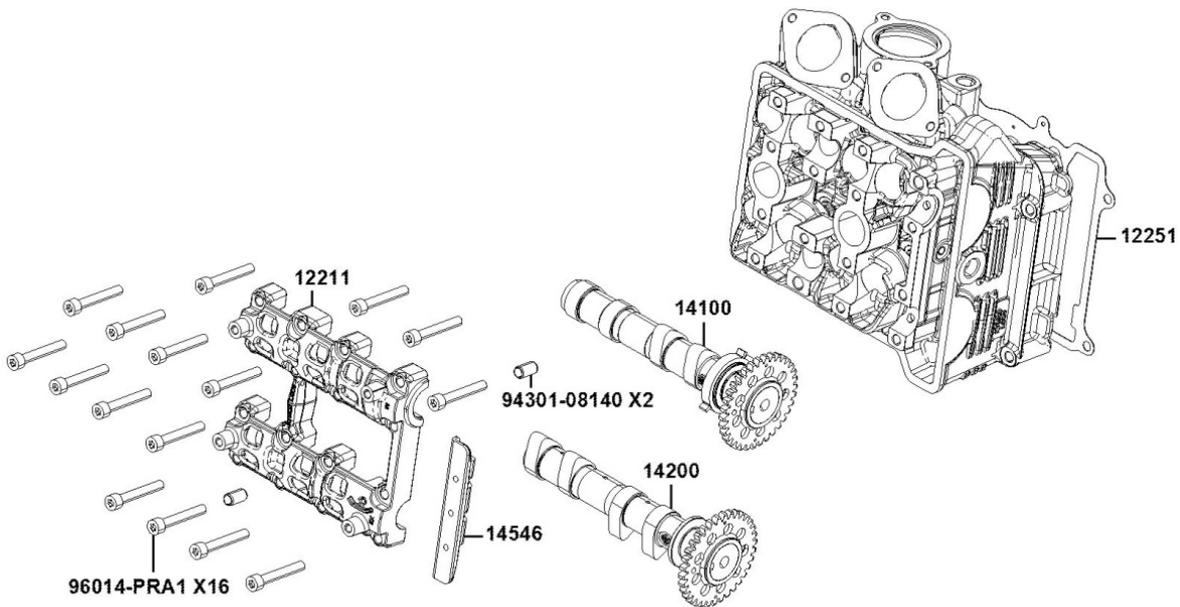
The camshaft holder and cylinder need with the same number mark.
