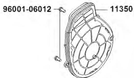
Remove the bolts, nut and remove the CVT cover.
