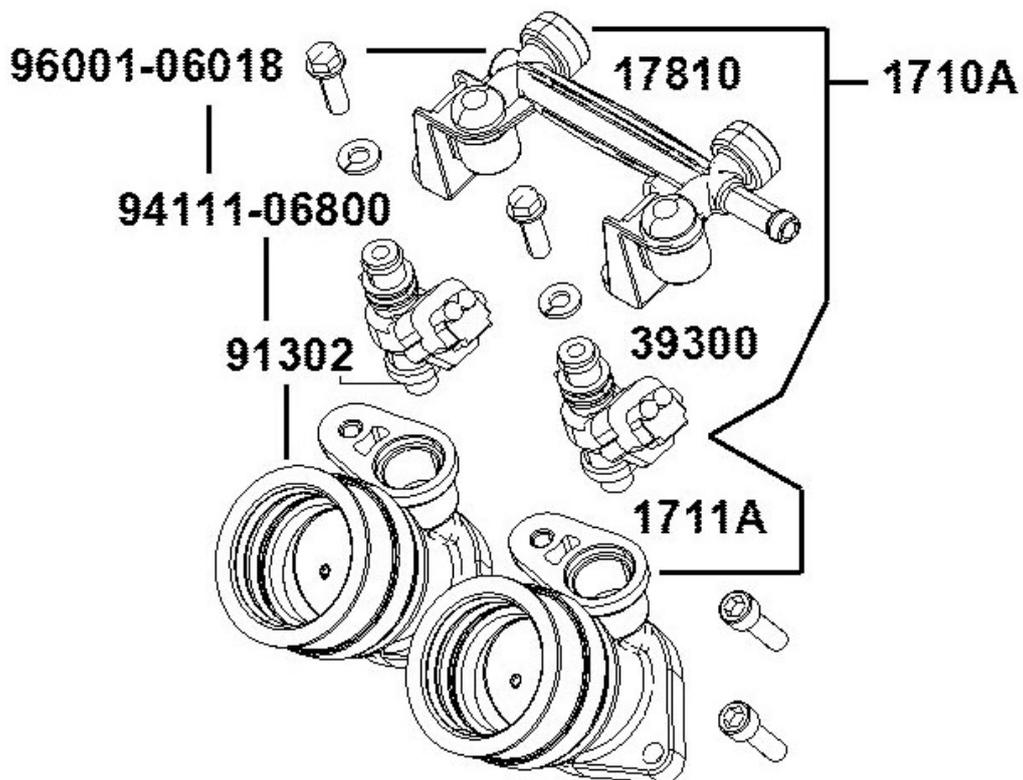
Fit the fuel injector pipe onto the top of the injector. The injector must securely fit into the pipe.
