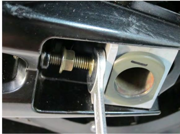
Remove the two bolts and remove the rear cushion.
