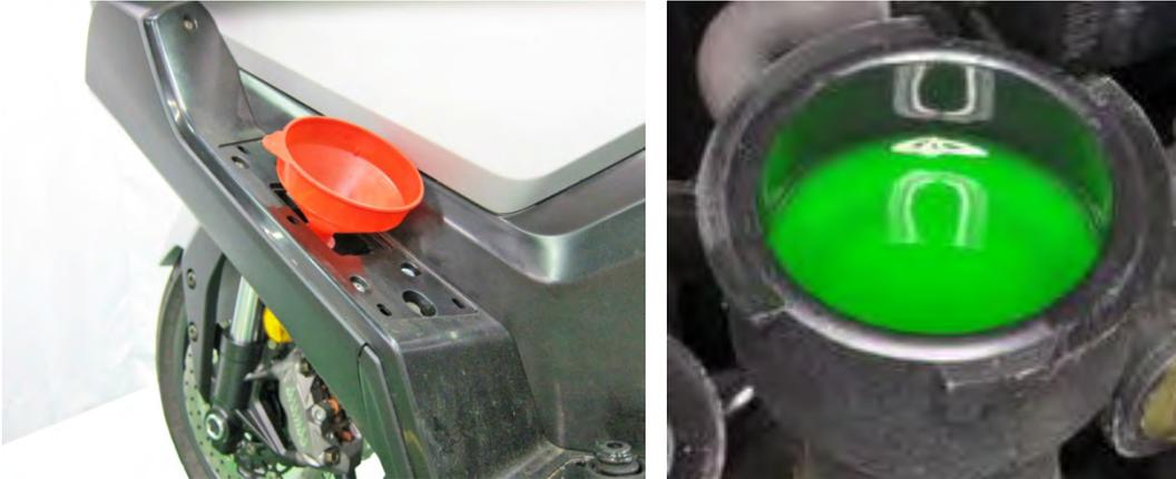
When the air bubbles stop coming up turn off the engine and recheck the coolant level, add coolant if necessary. Check the reserve tank and add coolant if needed. Wet the seal of the radiator cap and install.
