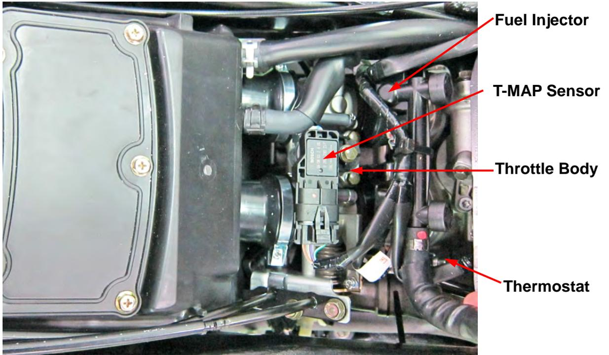
Loosen the two screws of throttle body/air cleaner clamps.
