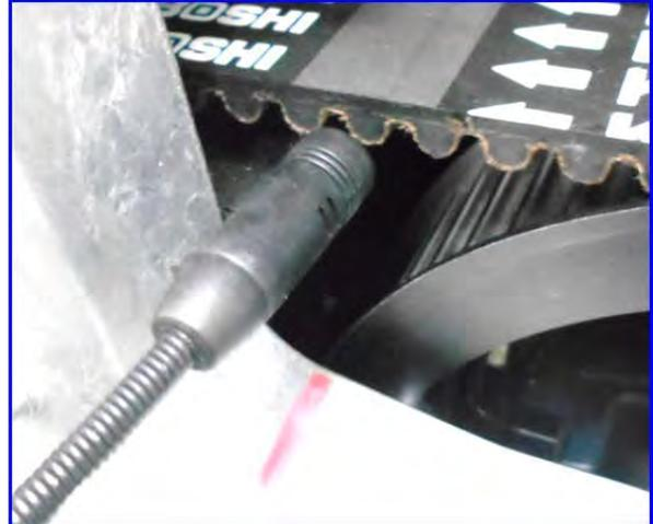
~1. Probe of Sonic Tension meter should be parallel to the belt as shown above pictures.
