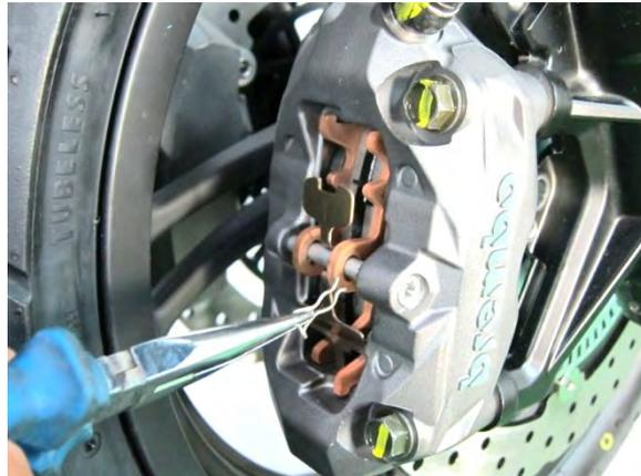
Remove the screw, loosen the brake pad.
