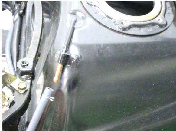
Remove the fuel tank mounting nuts.
