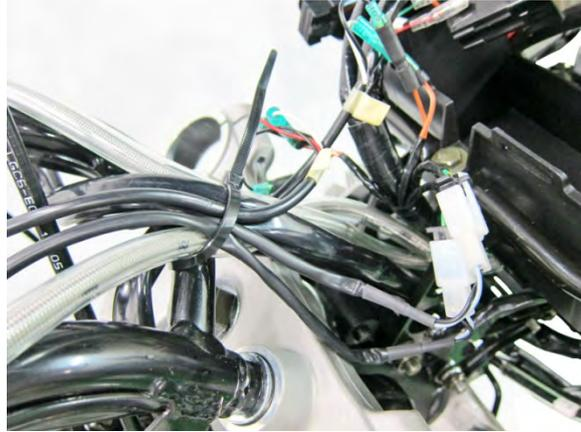
Disconnect the connectors and couplers of the switches.
