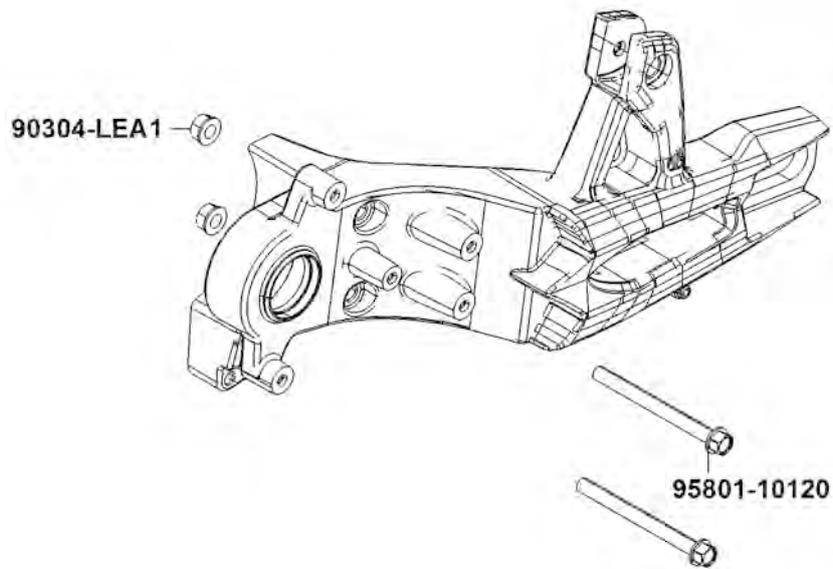
Remove the two dowl pin of the rear fork.
