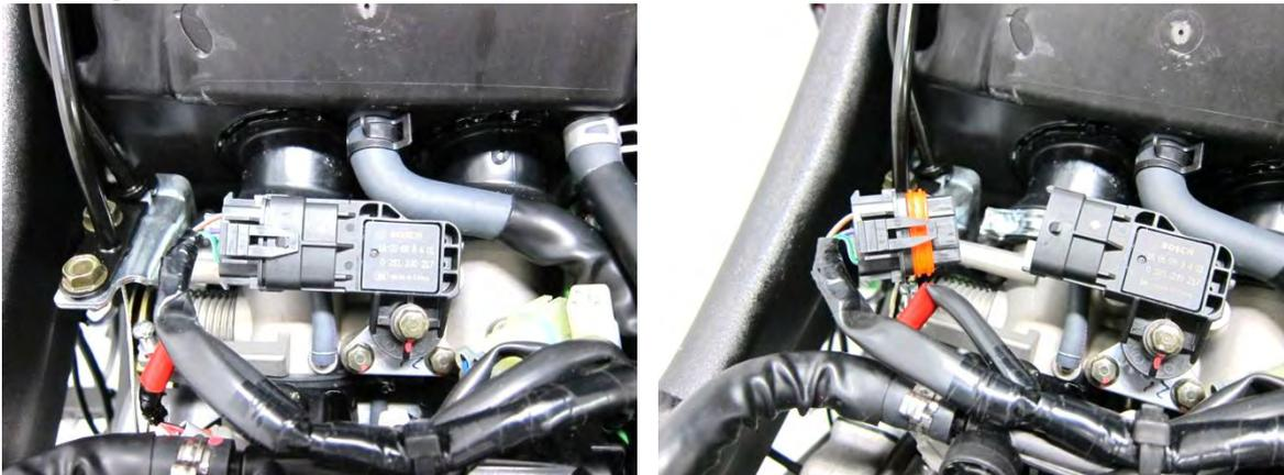
Measure if the ECU voltage outputs to the MAP between the following terminals of the MAP connector.
