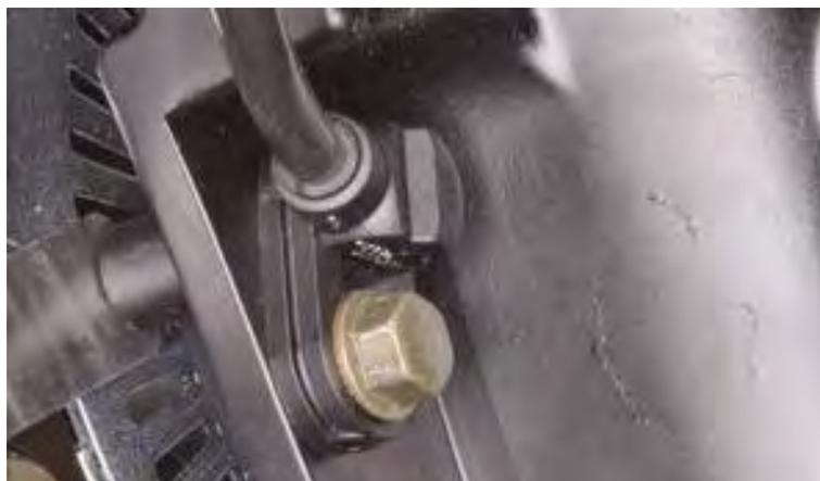
Check the speed sensor to rotor clearance with a feeler gauge and make sure that it is 0.3 - 1.2 mm (0.0012 - 0.048 in).
