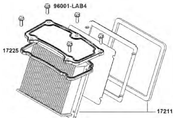
The new air cleaner element set installation is in the reverse order of removal.
