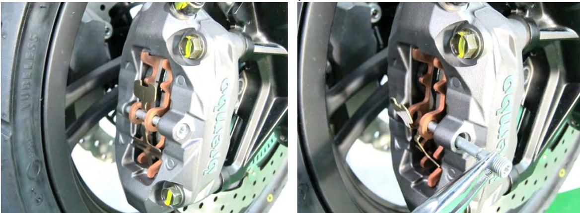
Remove the spring of the brake pad.
