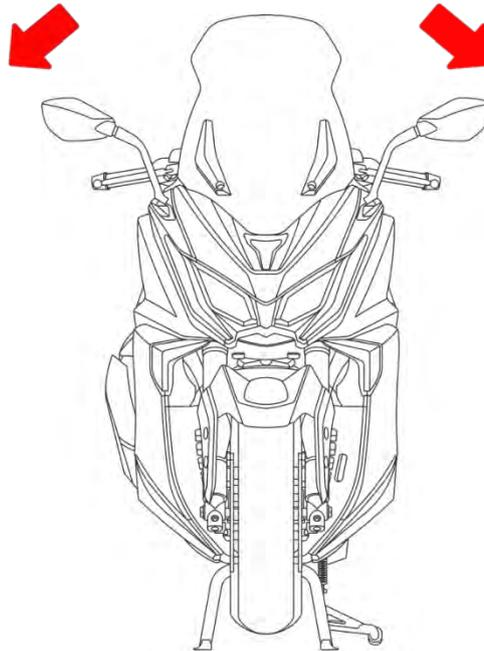
Raise the front wheel off the ground and check that the steering handlebar rotates freely. If the handlebar moves unevenly, binds, or has vertical movement, adjust the steering head bearing. See the Steering Stem Removal topic for more information.
