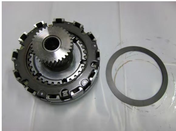
Remove the retainer and brake shoes set.
