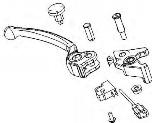
Remove the two master cylinder mounting bolts with an 8 mm socket.
