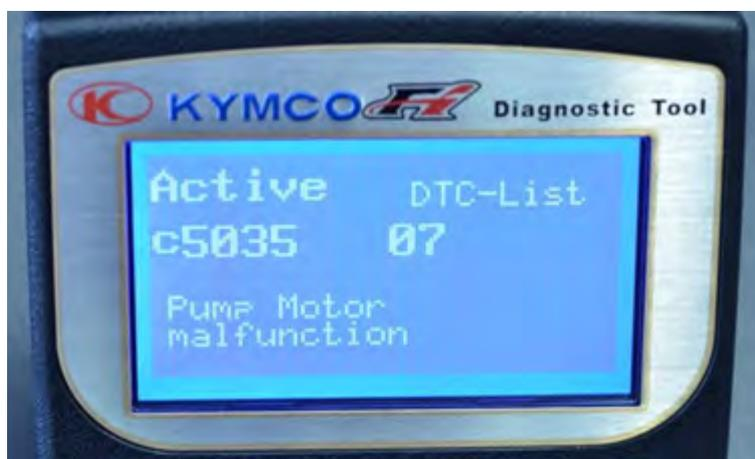
Check and clear the ABS DTCs in the same manner as the fuel injection DTCs.
