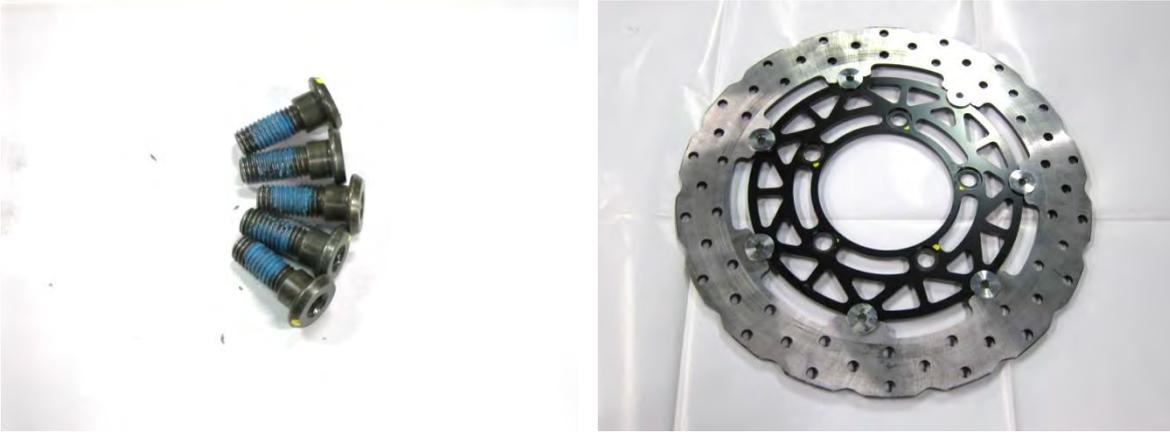
When installation, follow the order below, first time tighten the bolts with torque: 1.5 kgf-m (15 N-m)
