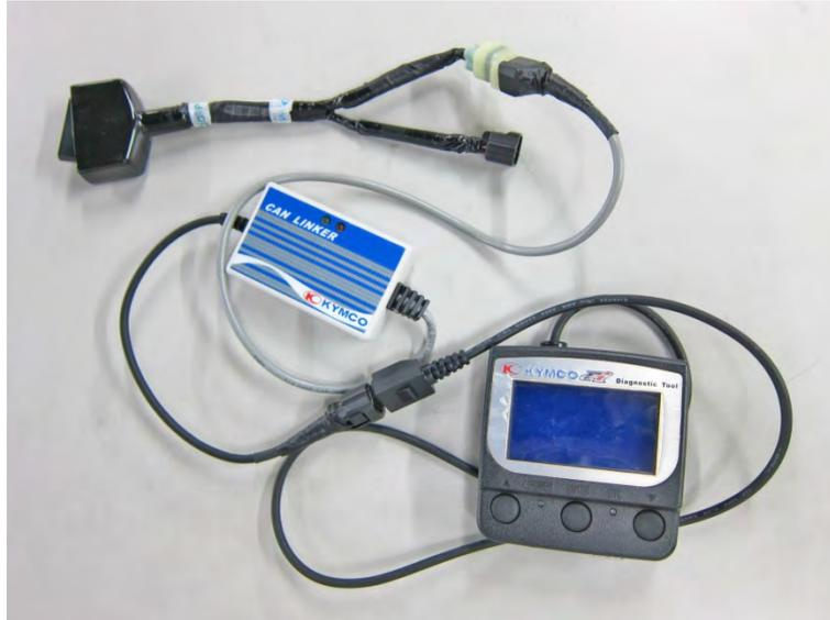
Plug in the tool to the ECU connector and turn on the ignition switch to send power to the tool.
