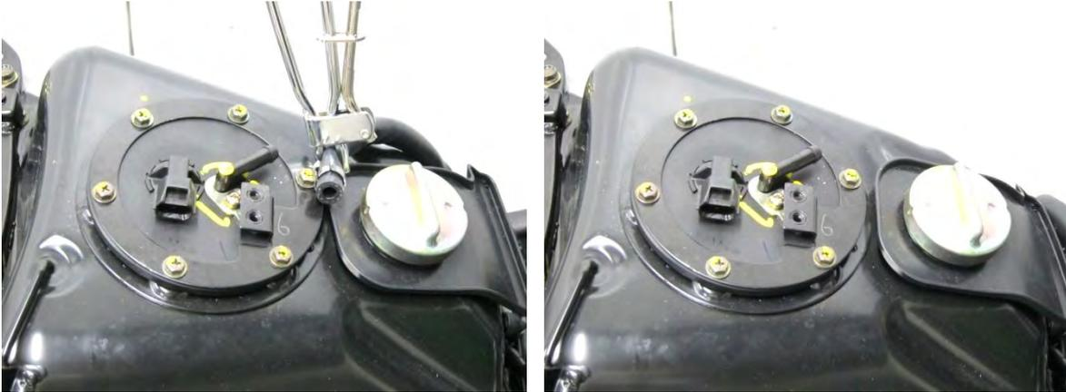
Note: When slide back the fuel hose carefully not to damage the fuel pump pipe, and replace the clamp with a new one when installation.
