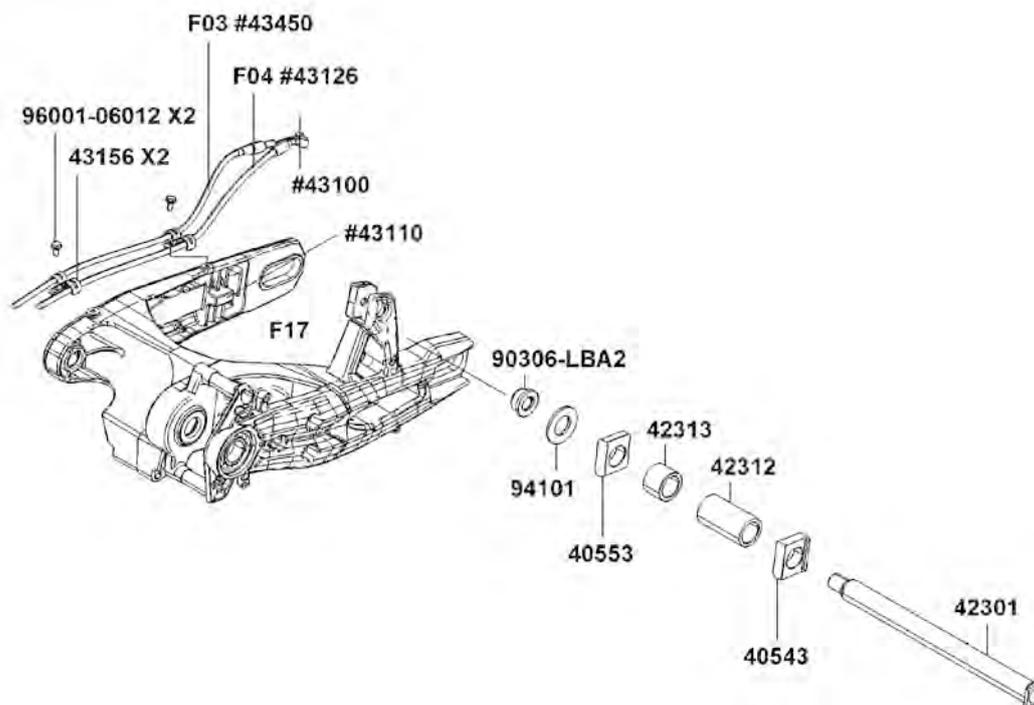
Loosen and remove the rear swing axle nut and washer.
