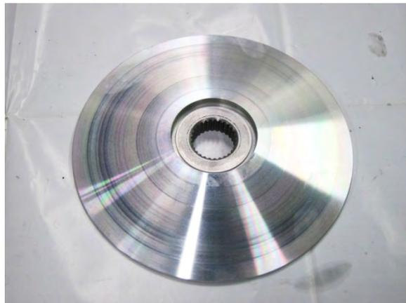
When installation, make sure the drive face are clean and grease free where they will contact the belt.
