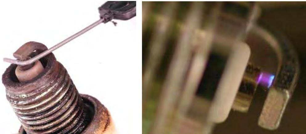
If the spark plug center electrode or side electrode are corroded or damaged, or if the insulator is cracked, replace the plug.
