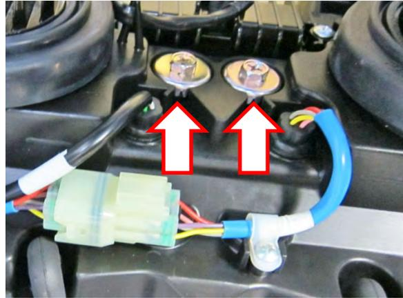
Turn the screws to adjust the right and left head lights aim as needed.
