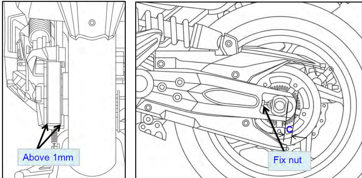
~1. Turn the wheel for several runs, check the belt is located at the center of driven pulley, (both sides clearance should be more than 1mm), if not, slightly adjust R/H Adjuster, and distance C of R/H and L/H Adjuster must remained within the range  $18.8\pm 0.5\text{mm}$ .
