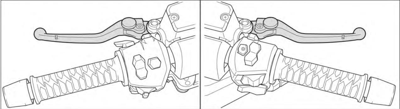
There is adjuster on each brake lever. Each adjuster has four positions so that the released lever position can be adjusted to suit the rider's hands. To adjust the distance of the lever from the handlebar grip, push the lever forward and turn the adjuster knob to align the number with the arrow mark on the lever holder.
