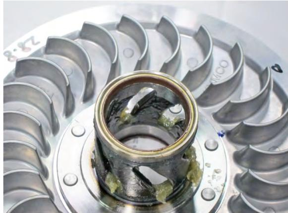
Replace the O-rings of the driven pulley.
