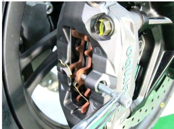
Remove the spring of the brake pad.
