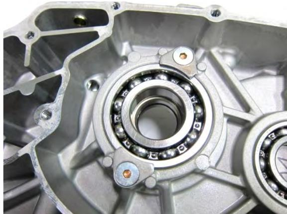
Remove the two bearing fixed plate.
