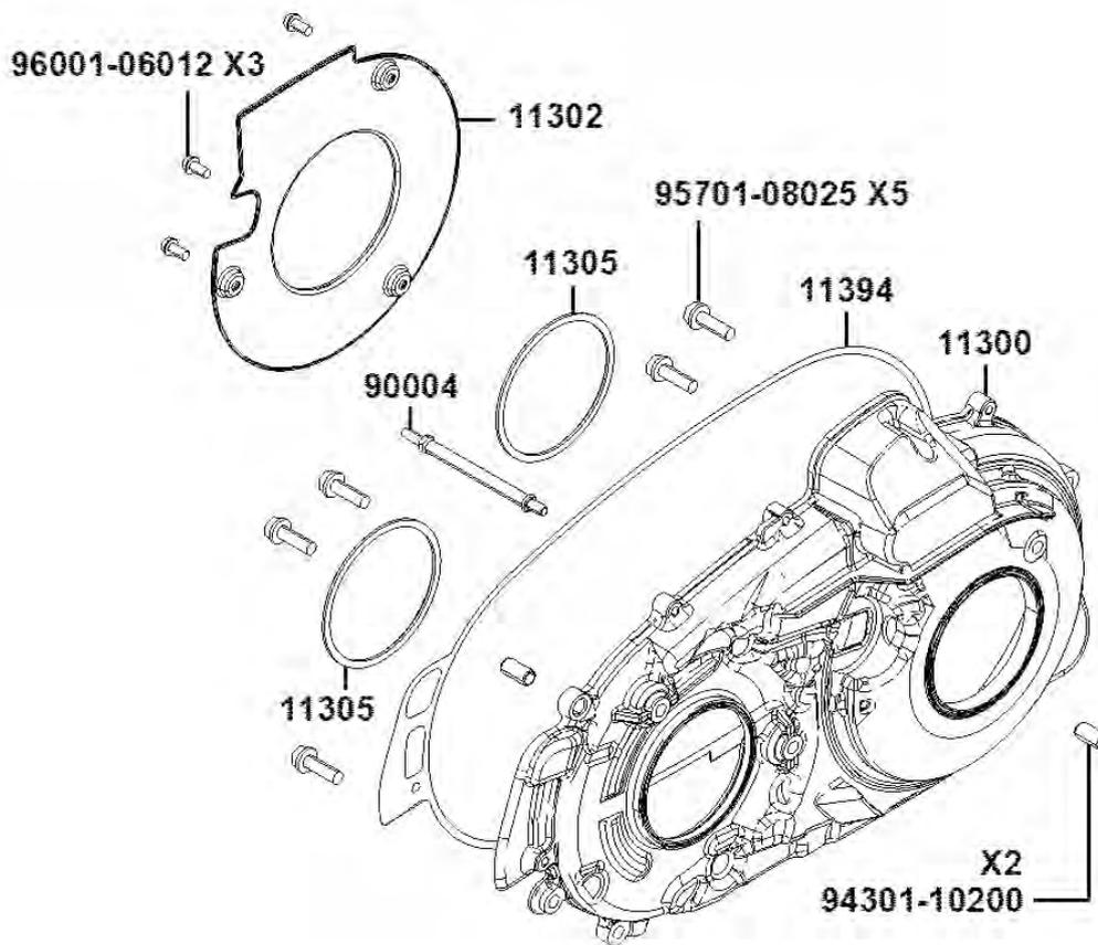
Driven Pulley Disassembly
