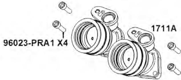
Slide back and remove the throttle body.
