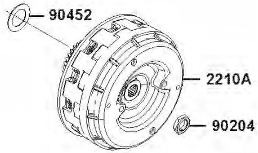
Wet Clutch Disassembly
