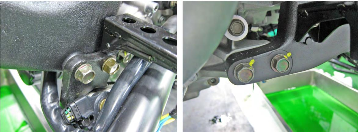
Carefully move the front frame forward and separate it from the engine.
