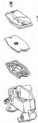
Clean and inspect the rubber diaphragm for tears or other damage. Replace as necessary.
