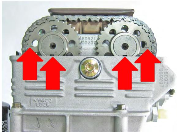
For correct engine timing the marks on the camshaft sprocket must be even with the cylinder head mating surface at the same time the "T" mark is lined up with the with the index notch in the timing inspection hole.
