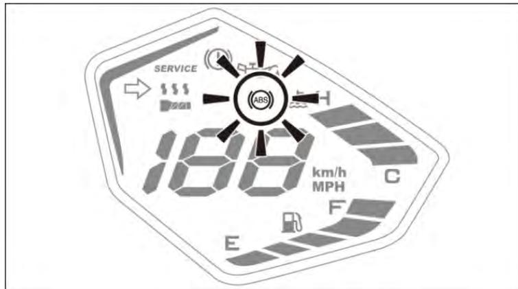
The ABS indicator light is on the left side of the meter. This light will come on when the ignition switch is turned on and goes off shortly after the vehicle starts moving. The light stays off as long as the system is ok.
