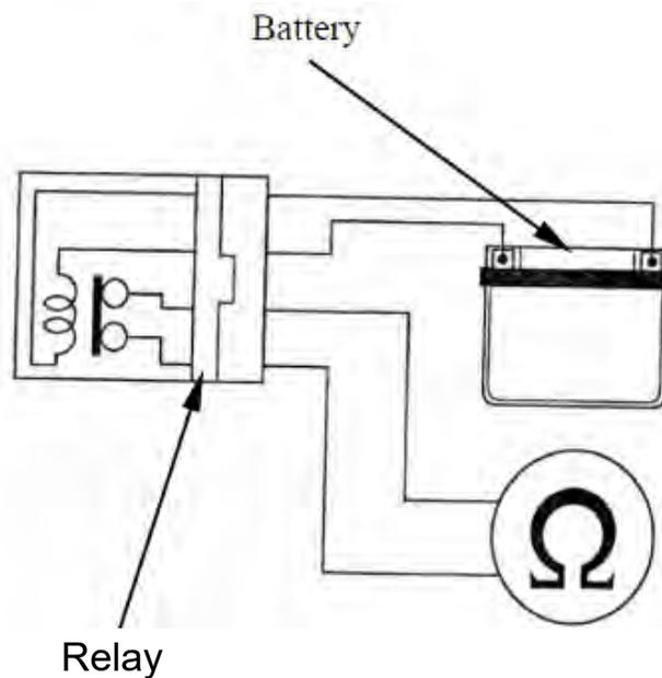
Connect 12 V battery with the fuel cut-off relay connector.
