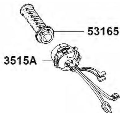
Disconnect the switches and heater connector.
