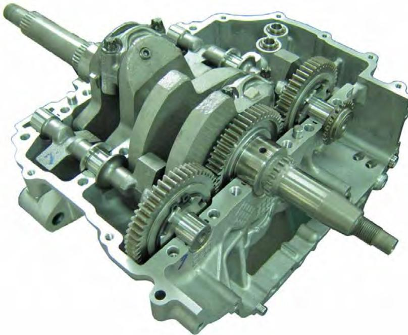
Install the crankshaft, balancer gears in the correct timing.
