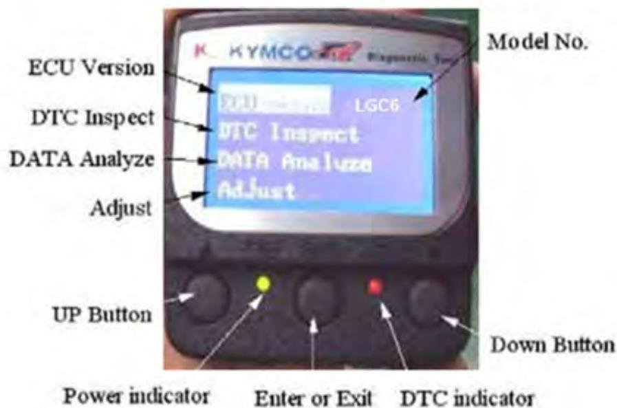
□ The functions of the diagnostic tool include ECU version, model name, data analysis and reset.
