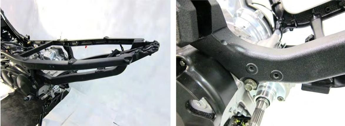
Remove the bolts and nuts and remove the rear frame body.
