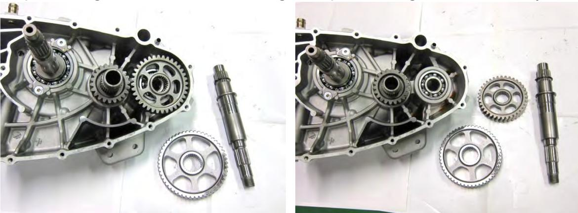
Remove the counter B gear and remove the counter gear.
