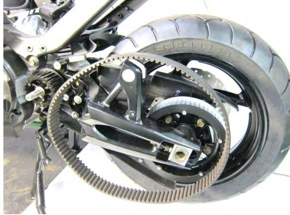
Remove the drive sprocket.
