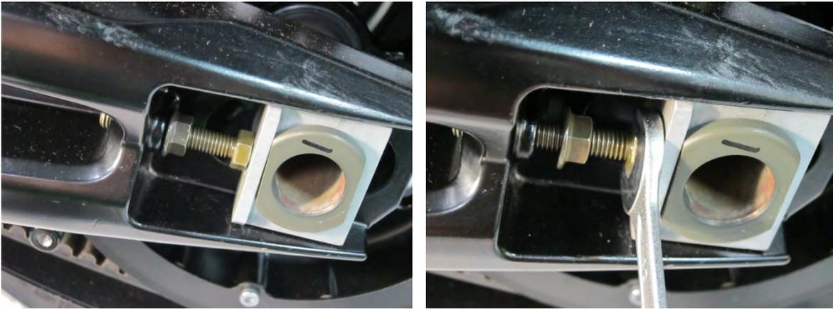
Remove two bolts and remove the chain up cover A.
