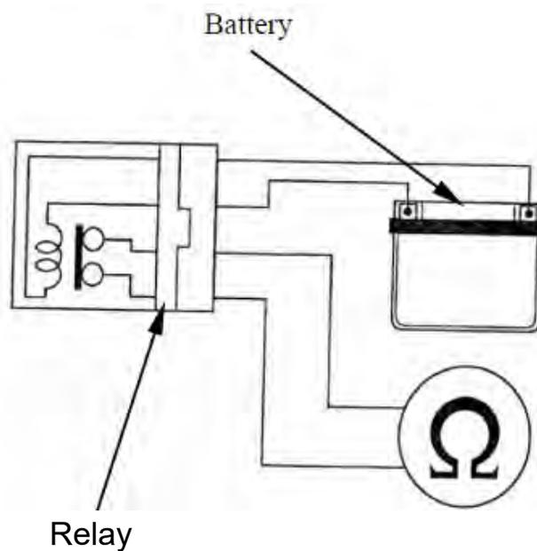
Connect 12 V battery with the fuel cut-off relay connector.
