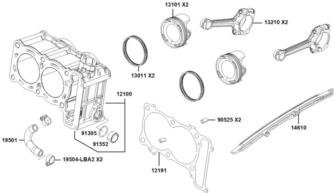
Remove the cylinder head gasket and dowel pins.
