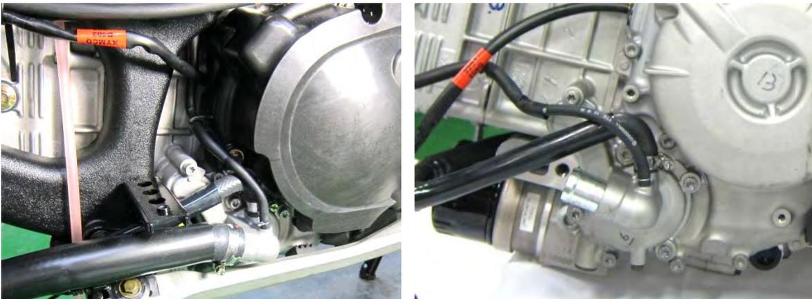
Remove the other coolant hose and tube. And remove the bolts of coolant pump cover.
