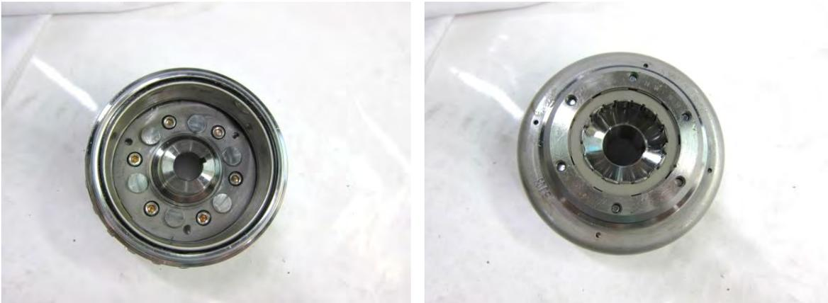
Remove the starting clutch gear.
