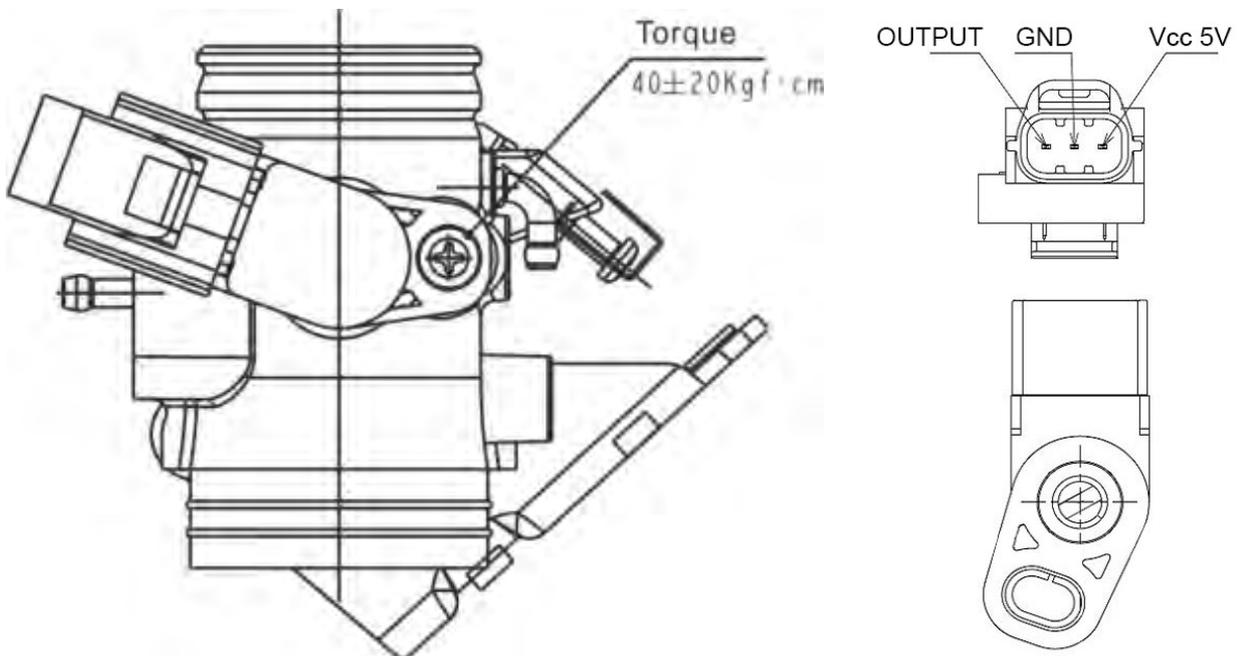
When installation, apply oil onto a new O-ring. Install the TPS onto the throttle body, being careful not to damage the O-ring. Install and tighten the screw securely.
