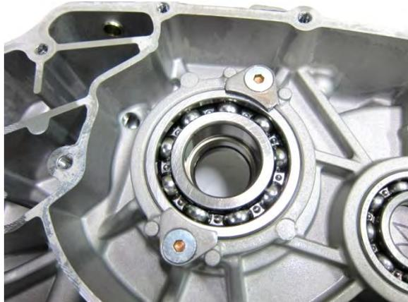
Remove the two bearing fixed plate.
