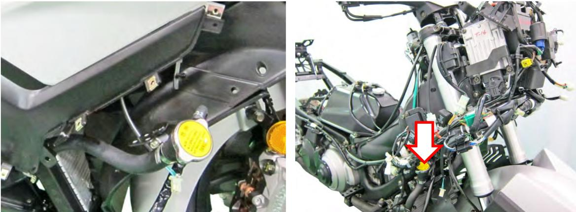
Remove the radiator cap in two stages. Allow any built up pressure to vent and then open the cap all the way and remove it.
