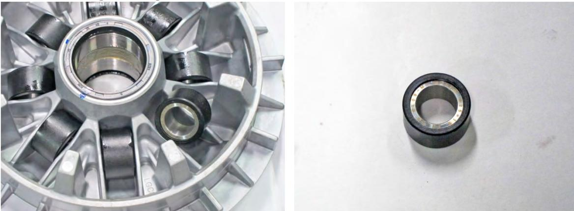
Remove the rollers and check them for excessive or uneven wear. Replace the weight rollers as needed.
