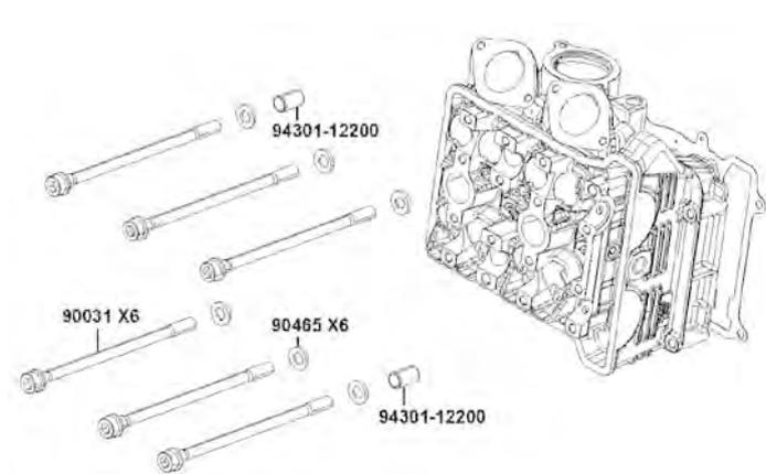
Remove the cylinder head gasket and dowel pins.
