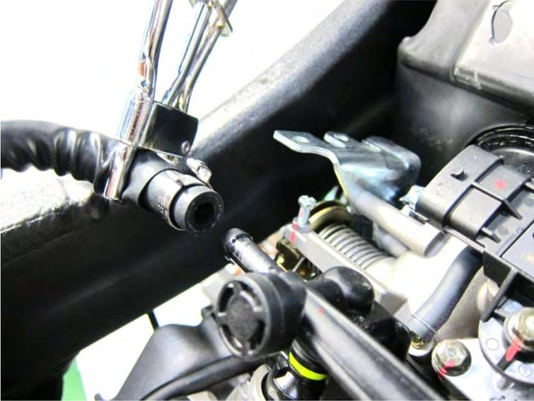
Remove the two fuel injector mounting bolt with a socket.
