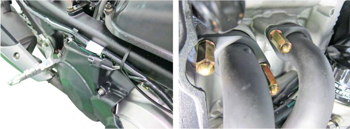
Remove the exhaust pipe.
