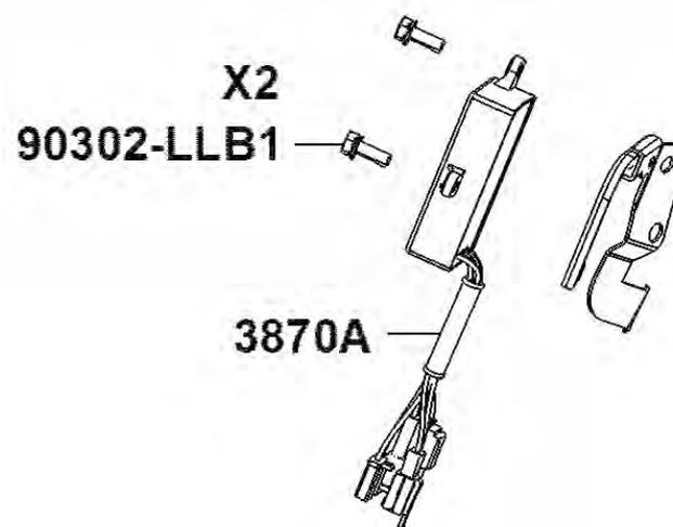
Remove the couplers and grip heaters replace the grip set if necessary.
