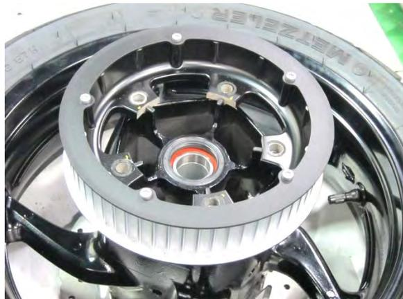
Remove the driven belt sprocket.
