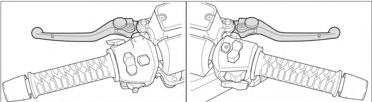
Use a digital multimeter to check for continuity to inspect the handlebar switches. Continuity should exist between the wires as indicated.
