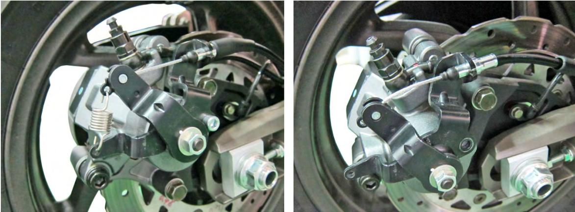
Remove the screws of handle bar switch, parking brake wire and remove the parking brake set.
