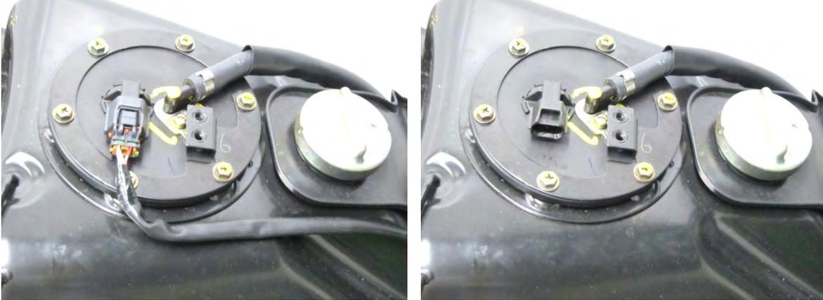
Touch the multi meter leads to the harness side of the fuel pump connector, with the positive lead touching the red/black wire terminal and the negative lead touching the green wire terminal.
