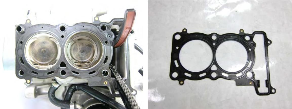
Remove the cylinder, gasket and dowel pins.
