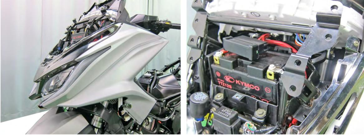
Remove the screws and remove the front cover set.
