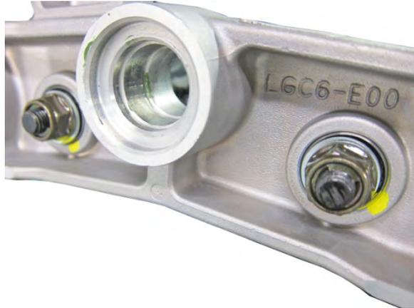
Remove the nuts and washer to separate the handle bar assembly.
