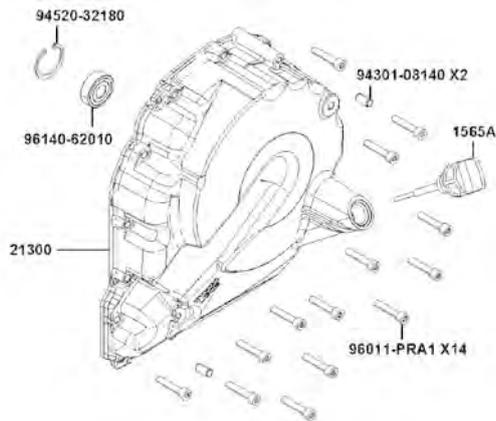
Remove the clip and check the bearing for wear or damage.
