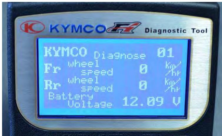
When using the DATA Analyze feature of the diagnostic tool with the ABS system the front and rear wheel speed sensors should show speed when the wheels are rotated.
