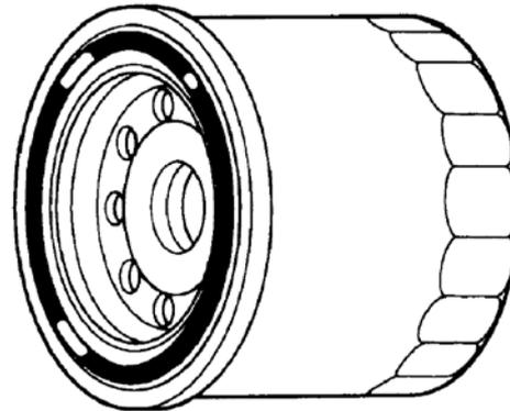
Make sure the O-ring is positioned correctly in the groove of the oil filter cartridge.
