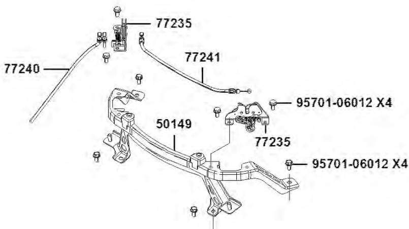
Remove the bolt, nut and collar of rear frame body.
