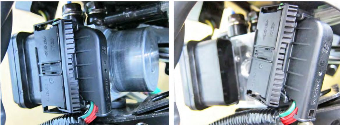
Disconnect the ABS hydraulic unit connector.
