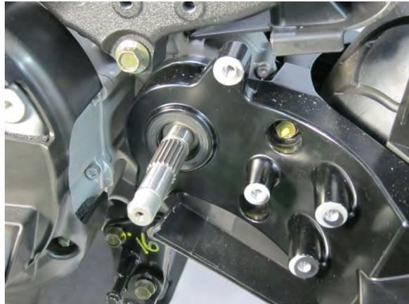
Slide out and remove the rear wheel axle.
