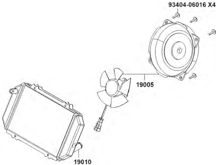
Inspect the radiator fins for damage and clogging. Clean out the fins with low pressure compressed air and water. Check the radiator for any bent or damaged fins. Use a small flat blade screwdriver to straighten them out, but be careful not to puncture the radiator.
