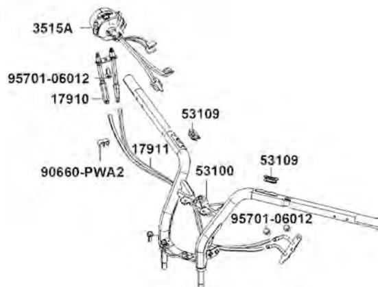
Disconnect the throttle cables and free the right switch housing from the handlebar. Separate the switch housing from the handlebar.
