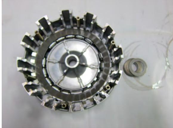
Remove the spring and lower retainer set.
