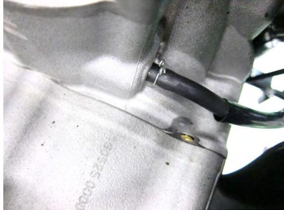
Loosen the two bolts of thermostat cover.
