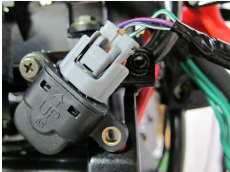
Incline the tilt switch  $65 \pm 10$  degrees to the left or right at the ignition switch “ON”. Measure the voltage as below.
