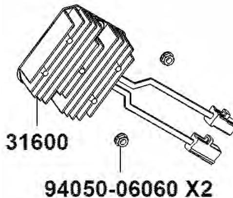
Disconnect the regulator/rectifier connector. Check the connectors for loose contacts or corroded terminals.
