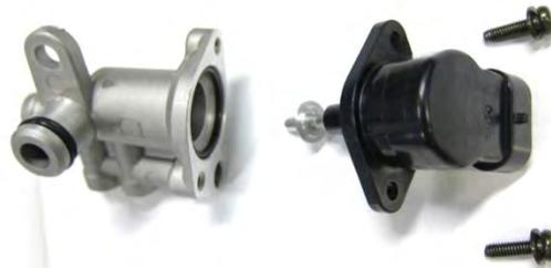
When installation, apply oil onto a new O-ring. And being careful not to damage the O-ring.
