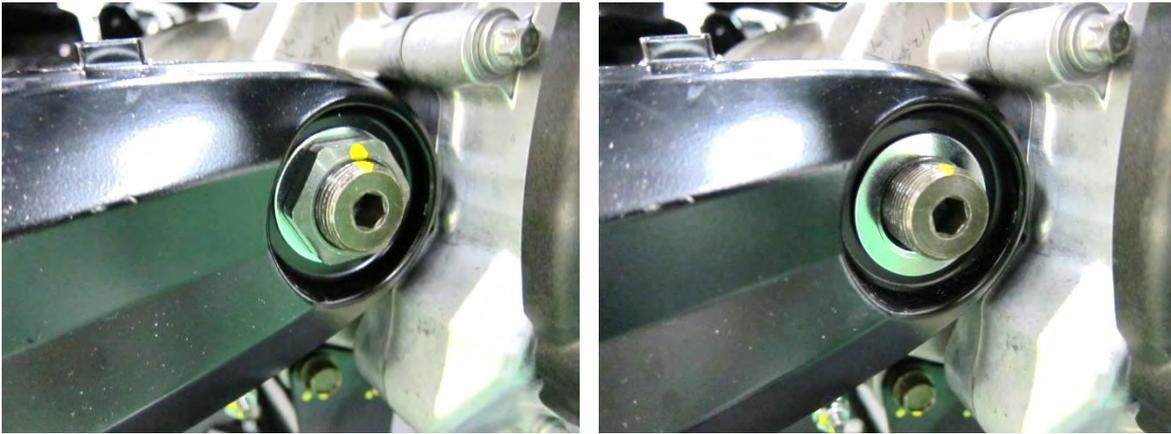
Loosen the rear swing axle bolt.
