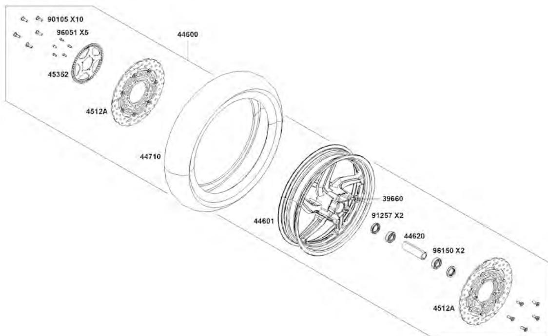
Loosen the front axle pinch bolt with a 6 mm Allen. Inspect the wheel speed sensor and brake disc for wear and damage. Replace the parts as needed.
