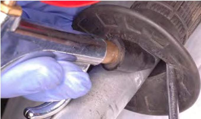
If you plan to replace the grips you can slice them lengthwise with a razor blade and peel them off. To remove the grips without cutting them use a screwdriver to open a gap between the grip and the handlebar. Spray in contact cleaner to break up the grip cement. Use compressed air to expand the grip so it can be easily slid off the end of the handlebar. Note the relationship between the angle of the grip and the throttle tube so that the new grip can be installed with the correct angle.
