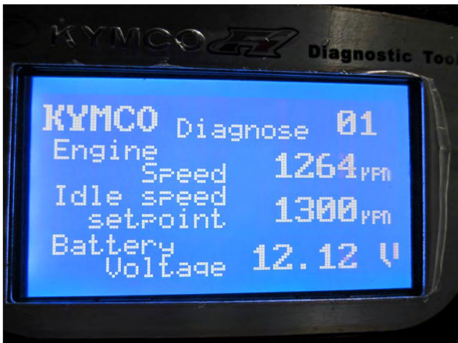
The 01 page shows engine speed, idle speed set point, and battery voltage.
