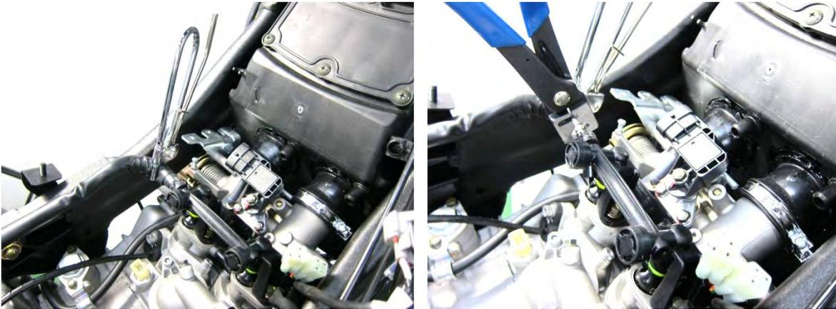
To separate the fuel hose from the fuel pump pipe.
