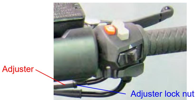
Loosen the throttle cable adjuster lock nut and turn the adjuster to achieve the specified free play.
