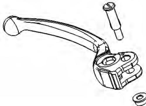
Unplug the brake light switch connector. Remove the lever and brake light switch.
