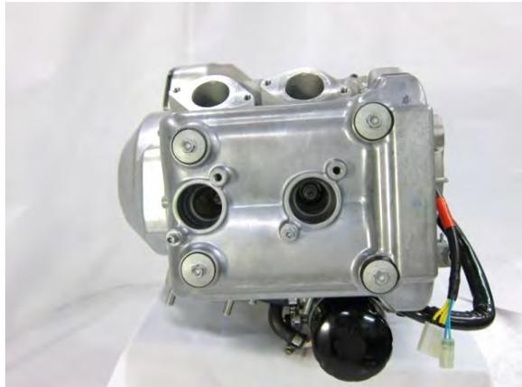
Remove the cylinder head cover. Replace the rubbers when installation.
