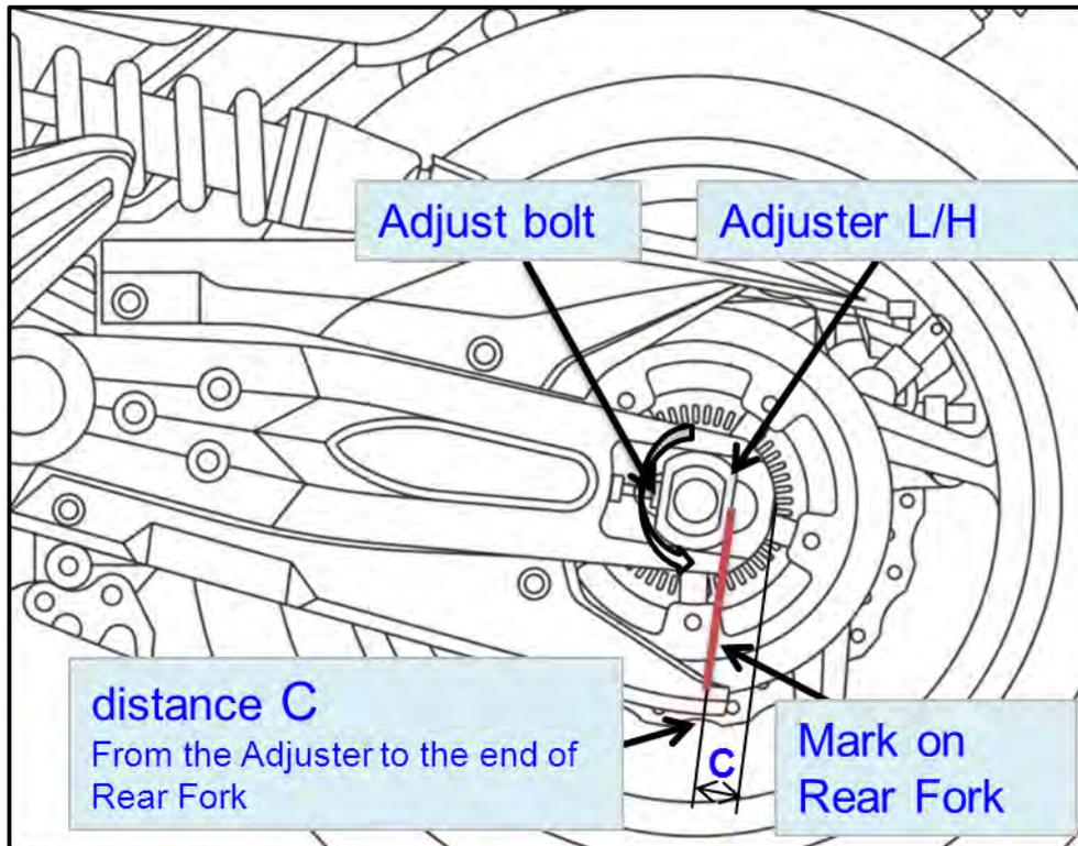
~1. Adjust L/H Adjuster place to the Mark on Rear Fork.
