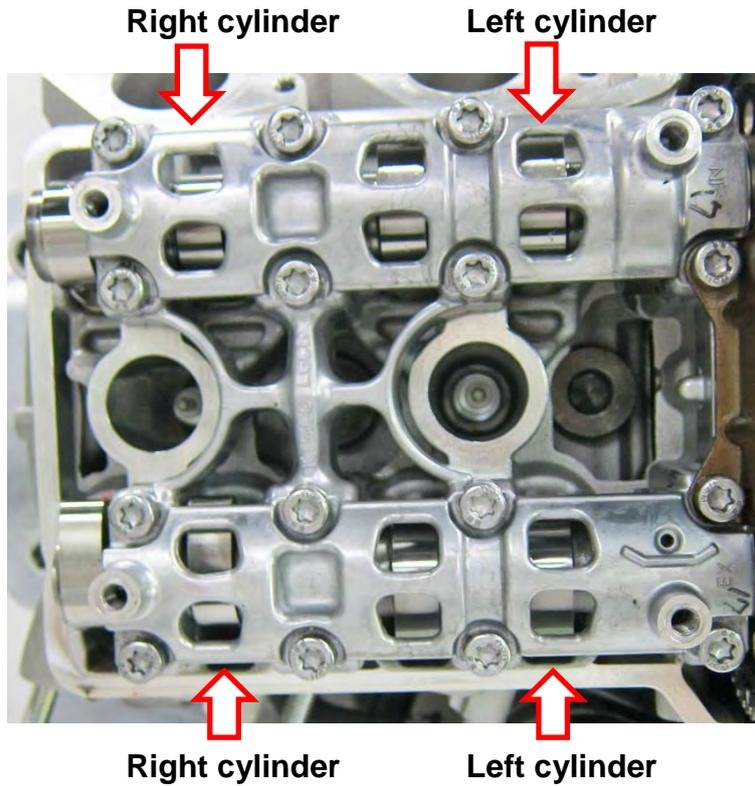
Measure the valve clearance with a thickness feeler gauge.
