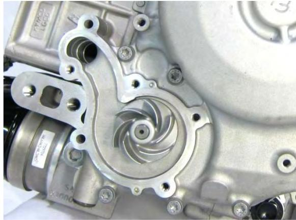
Remove the generator cover. See the [A.C. Generator and Starter clutch](#) topic for more information.
