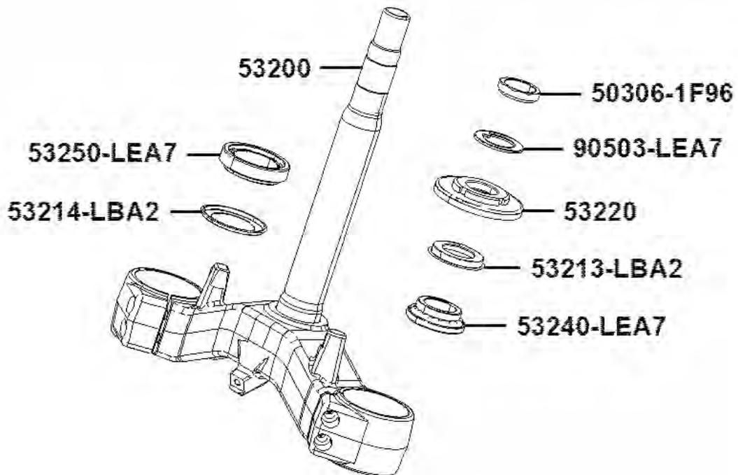
Use a chisel and hammer to drive out the bearing races. Do not damage the frame pipe and steering stem.
