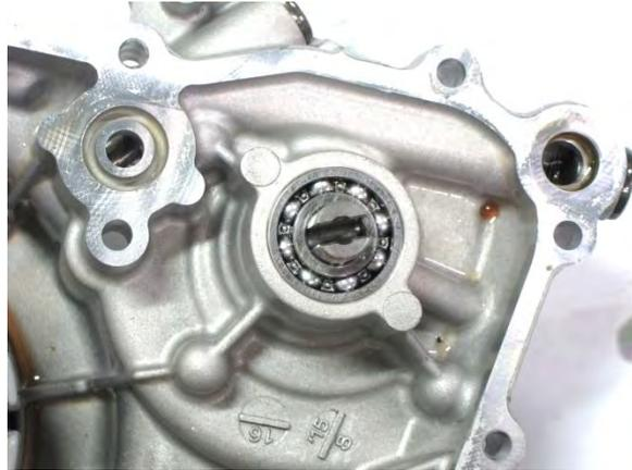
Remove the water pump shaft and impeller
