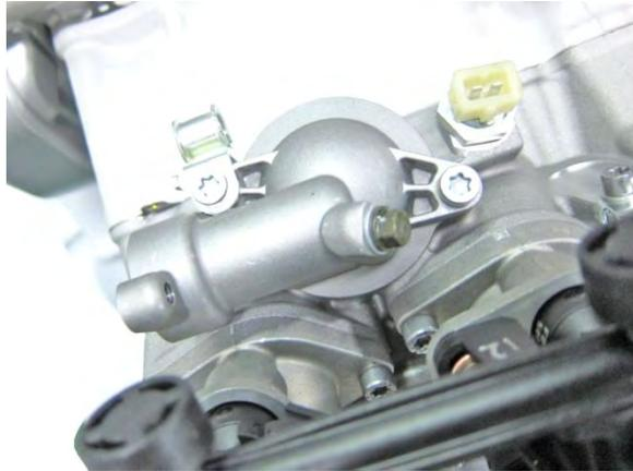
Use a 17 mm wrench to remove the water temperature sensor.
