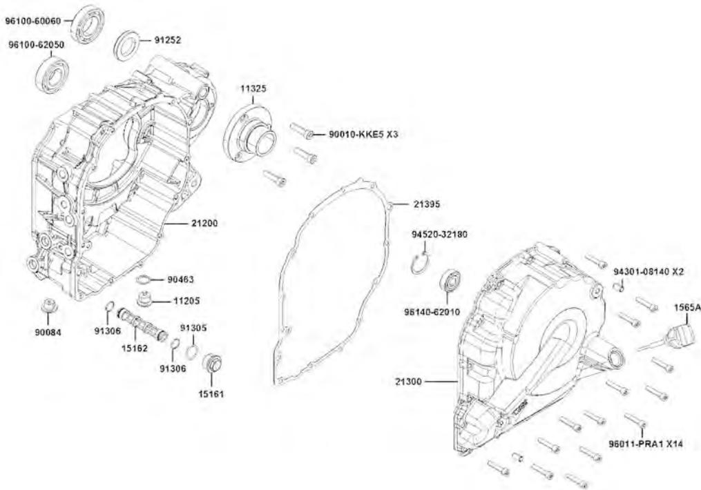
Remove the filter plug bolt and remove the filter.
