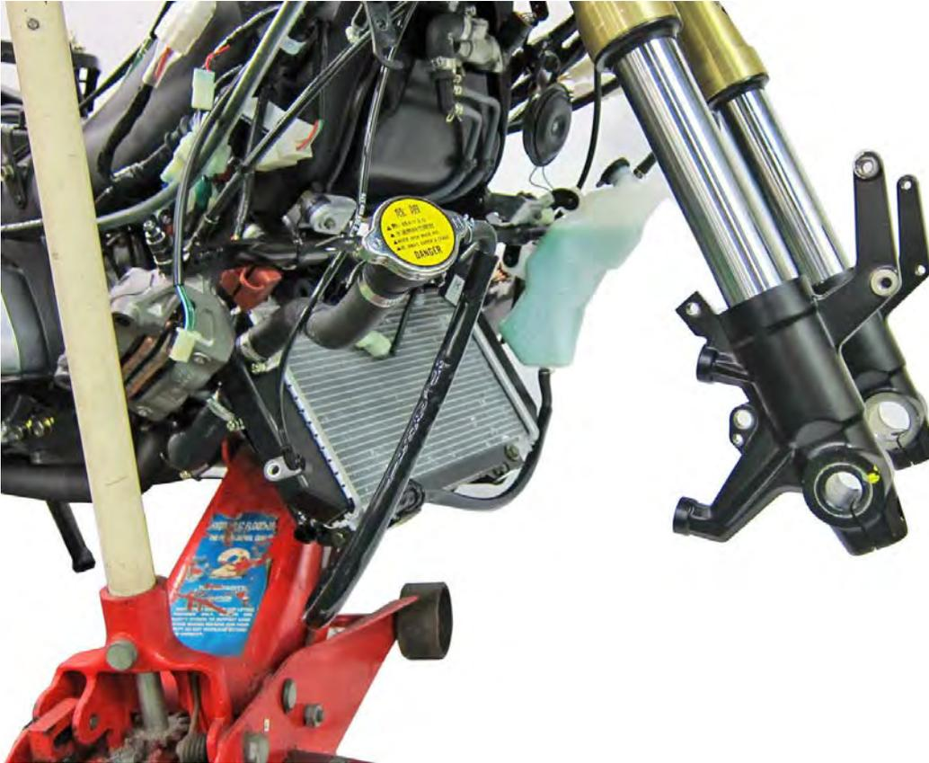
Support the vehicle with a suitable stand or jack so that the front wheel is off the ground. Grip the bottom of the fork legs and turn the front end side-to-side. If the movement is rough the bearings should be greased or replaced. If the movement is too tight or loose the steering stem adjusting nut may need to be adjusted.
