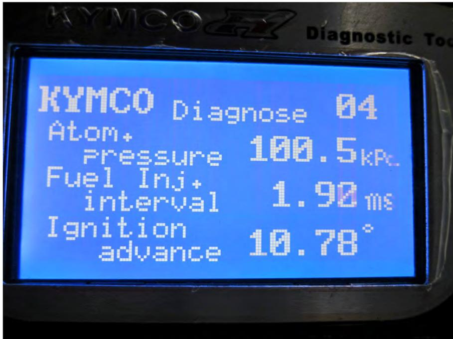
The 04 page shows atmospheric pressure, fuel injection interval, and ignition advance.
