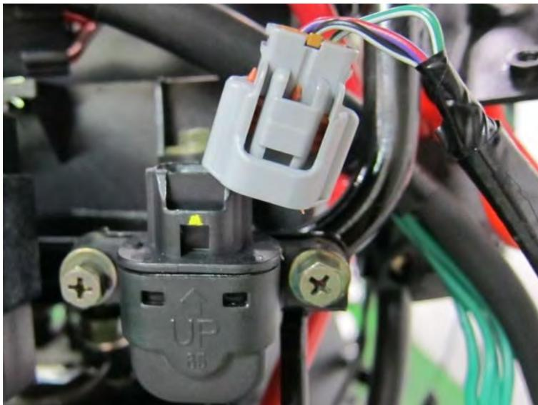
Disconnect the connector to remove the tilt switch.
