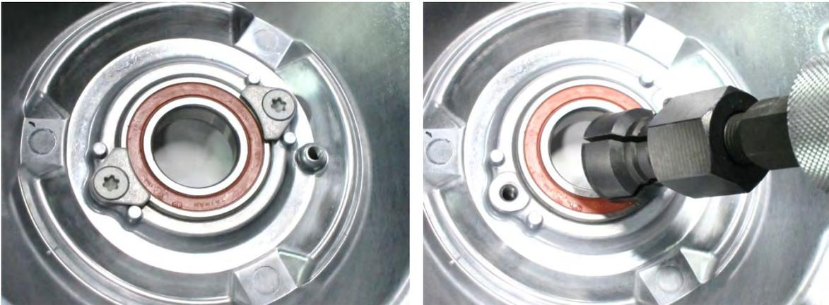
Drive in a new bearing with a suitable bearing driver that has the same outside diameter as the bearing.
