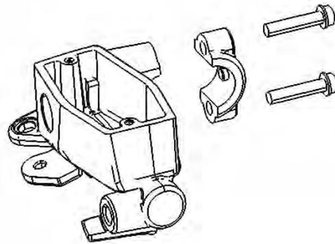
Be sure to insert the pin on the clamp into the hole on the handlebar when installation.
