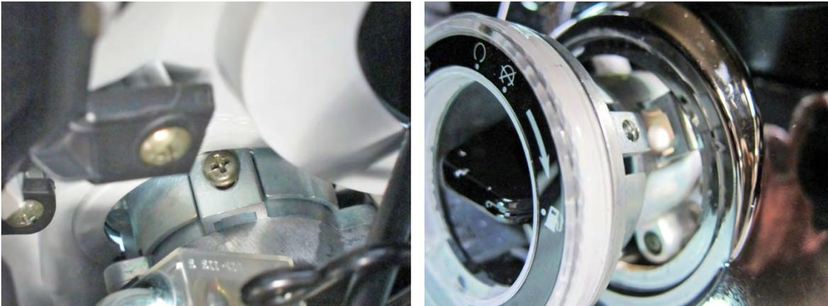
Remove bolts, screws, couplers and remove the leg shield assembly.
