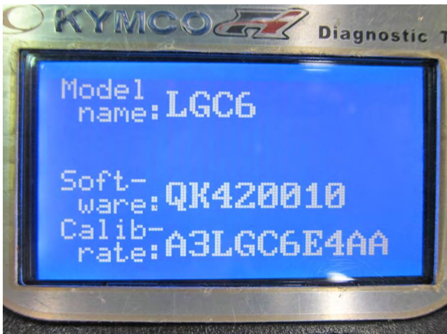
Pressing the enter button on the ECU version will show model name, ECU number, identifications number and software version.
