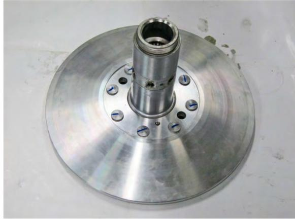
Replace the seals from the driven pulley.
