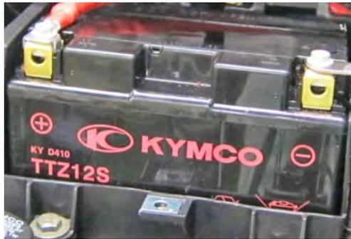
Check the battery voltage with a multi-meter. Place the positive probe onto the positive battery terminal and the negative probe to the negative battery terminal. If the battery reads under 12.3 V it is undercharged.
