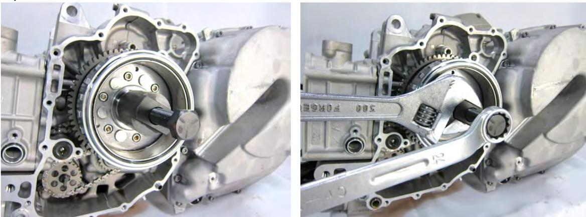
Inspect the one way bearing, replace if necessary.
