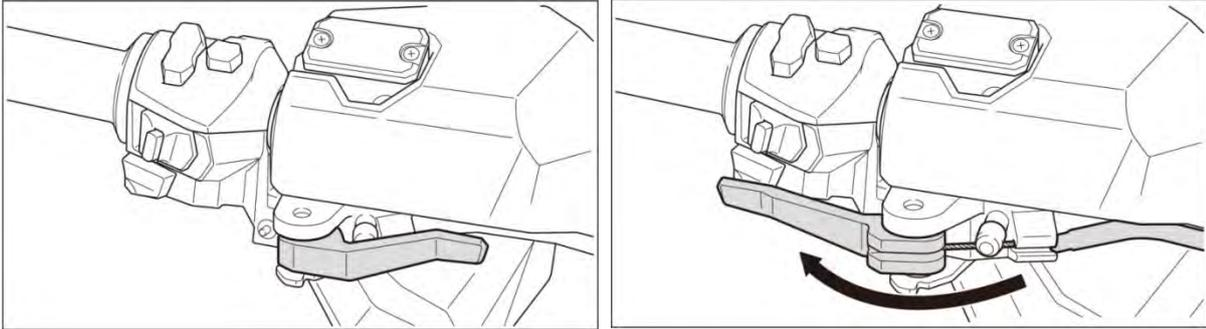
Release the fixed nut, and rotate the adjust nut to adjust the parking brake.
