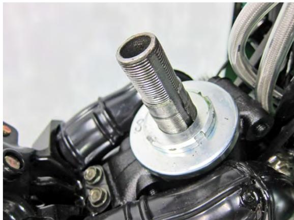
A special race nut wrench is needed to loosen the steering stem lock nut.
