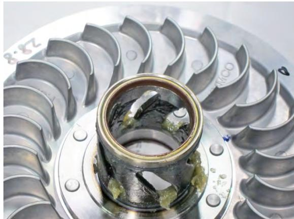
Replace the O-rings of the driven pulley.
