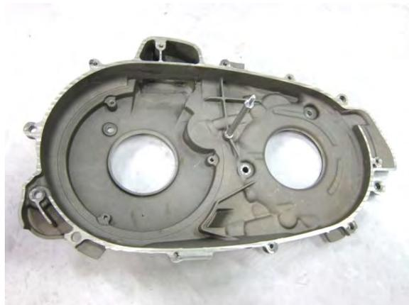
Remove the gaskets of CVT case.
