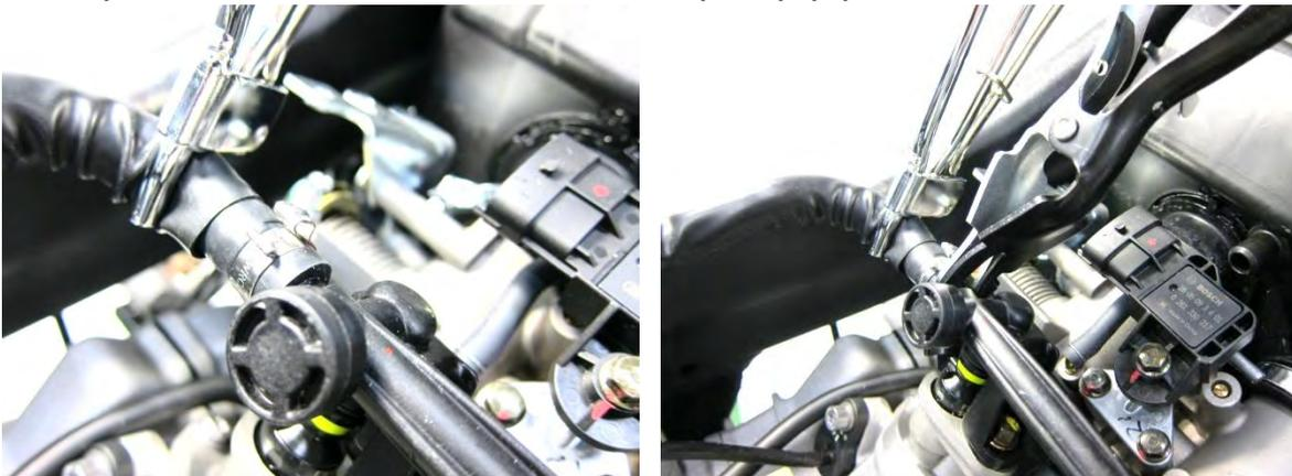
Slide back the clamp and free the injector fuel pipe from the fuel hose.
