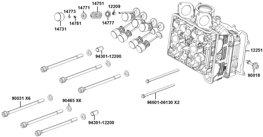
Remove bolts of cylinder head.
