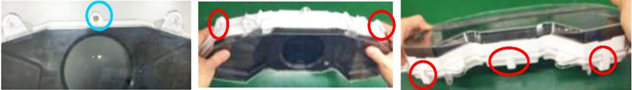
Remove the cover of meter. There is anti-fogging agent applied on the surface of inside cover.
