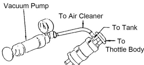
Connecting a vacuum pump to the tube of canister. (Follow the illustration below.)
