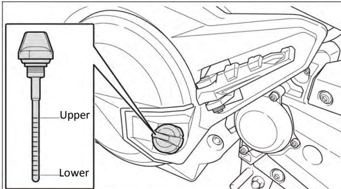
The oil filler cap/dipstick is located on the left side of the engine.
