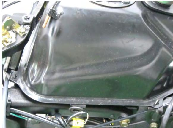
Remove the fuel tank mounting nuts and remove the fuel tank from the frame.
