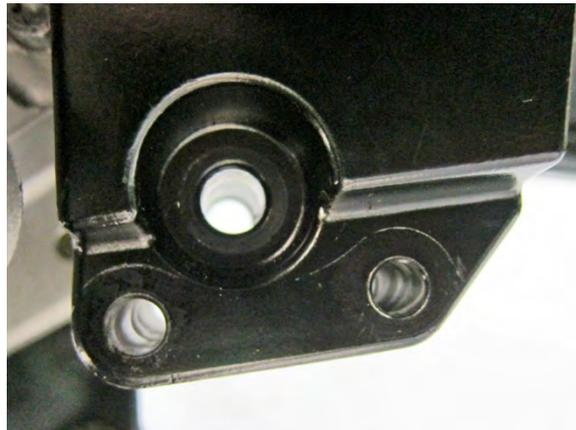
Loosen the two bolts of left rear fork.
