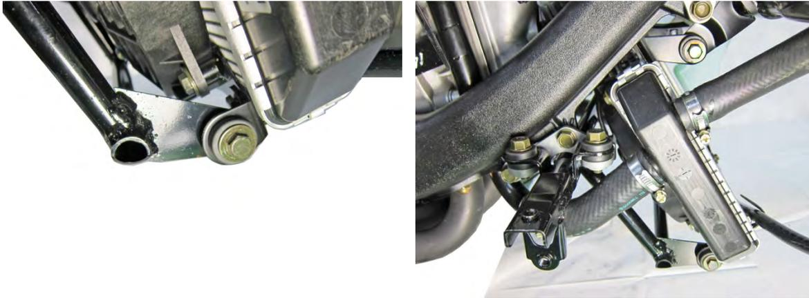
Remove the radiator and free the grommet from the radiator. And remove the tube and remove bolts of the fixed plate.
