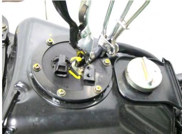
Clean up any remaining fuel immediately. Disconnect the fuel hose from the fuel injector. Connect the fuel pressure gauge. Remove the fuel hose clamp. Turn the key to the ON position. Check the fuel pressure.
