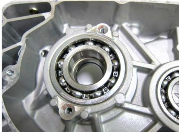
Remove the bearing by bearing puller tool.
