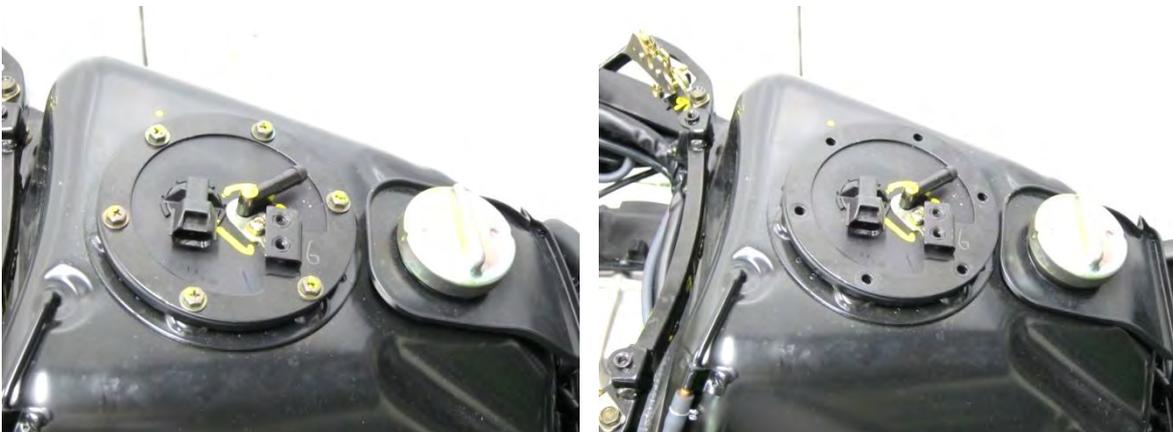
Remove the fuel pump assembly.
