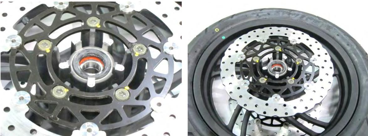
The bolts are all with blue Loctite (non-permanent) to the threads. Using this type of bolts when installation.
