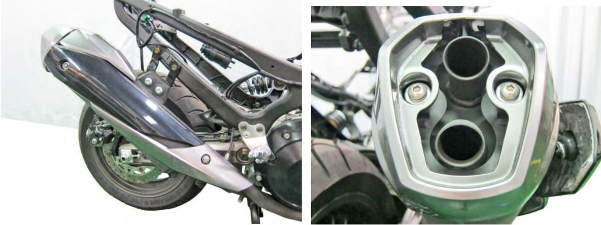
Remove bolts, washers, rubbers and remove the heat shields.
