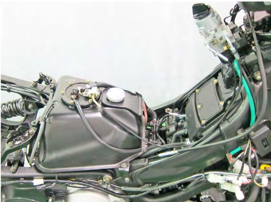
To remove the anti-tamper bolts use a punch and a hammer to strike the bolts so that they rotate loose. Turn the bolts clockwise to loosen them.
