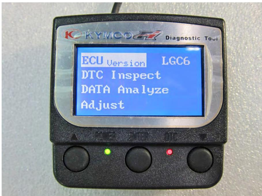
The four functions will display when the tool is powered on. The model name will show LGC6 for the AK 550.
