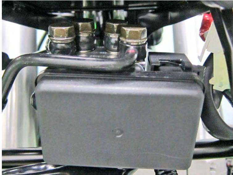
Note the markings on the ABS unit for the brake Front (F) and Rear (R) brake hose positions.
