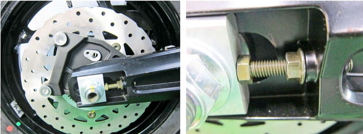
Loosen and remove the rear wheel axle nut, move wheel forward to loosen the belt. Installation torque: 12~14 kgf-m (120~140 N-m)
