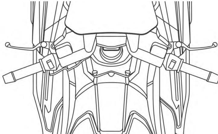
Pump the brake lever several times and hold the lever in. While holding the lever in, crack open the bleeder valve. The front brake lever will travel all the way to the grip and brake fluid and/or air will come out of the bleeder valve into the 6 mm hose. Tighten the bleeder valve before releasing the front brake lever. Pump the lever several times again and repeat the process.
