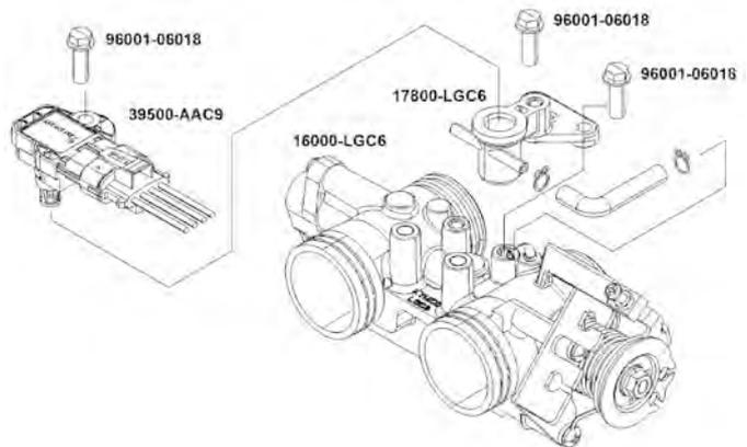
Remove four bolts of inlet pipe.
