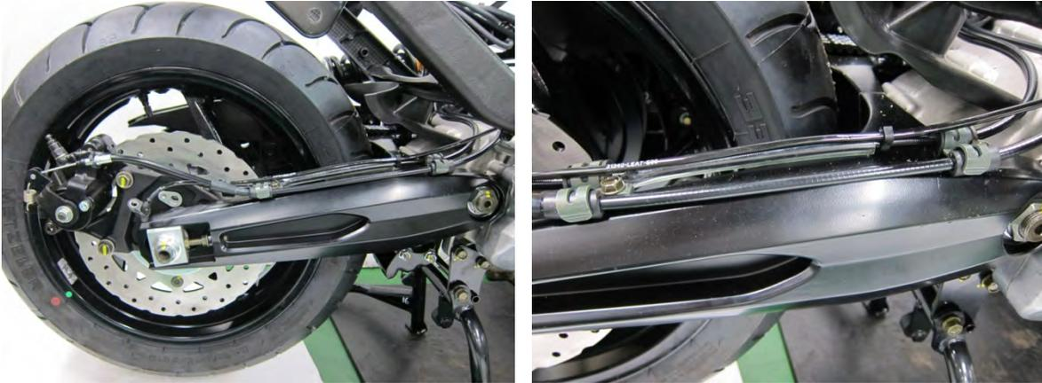
Remove the bolt of rear fixed plate.
