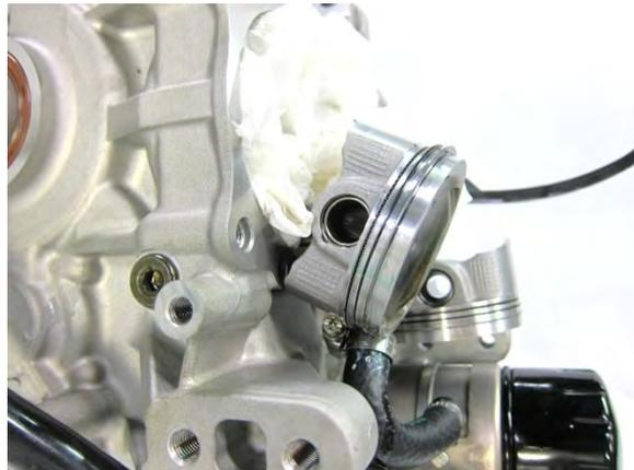
Remove the piston pin and the piston.
