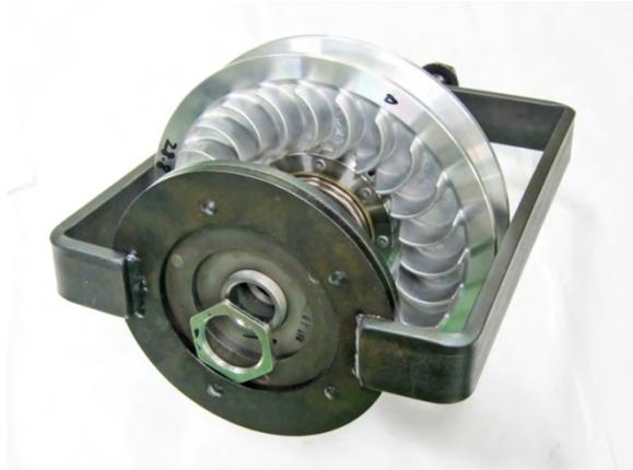
Loosen and remove the spring compressor tool.
