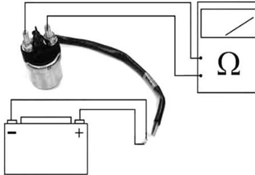
Check for continuity between the yellow/red wire and green/yellow wire. There should be continuity when the starter button is depressed. If there is no continuity, check the starter button for continuity and inspect the wire.
