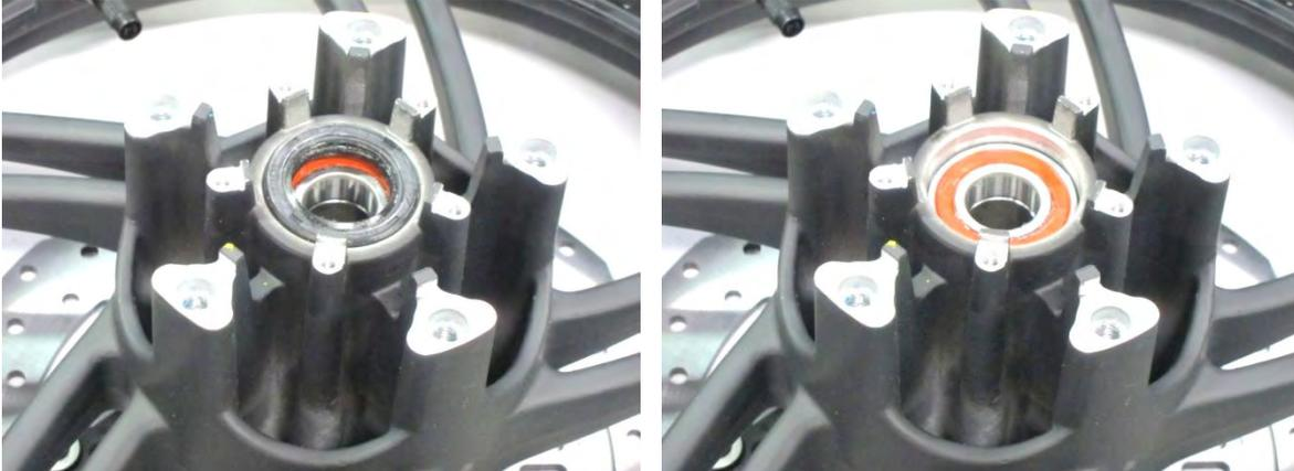
Remove the dust seal from the right side of the front wheel using a seal pick or large flat blade screwdriver. Discard the dust seal, it should be replaced by a new item.
