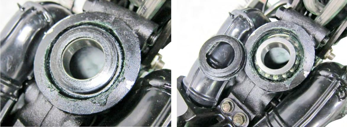
Remove the collar and remove the upper ball bearing.
