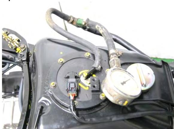
If the fuel output pressure is less than 3.0 bar, may fail to start the engine or in trouble in case of riding.
