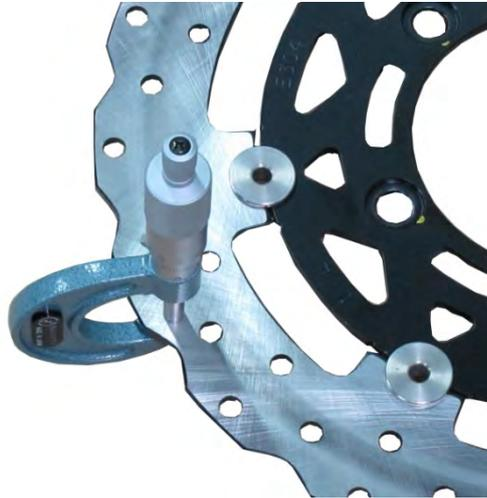
Measure the thickness of the brake rotor with a micrometer.
