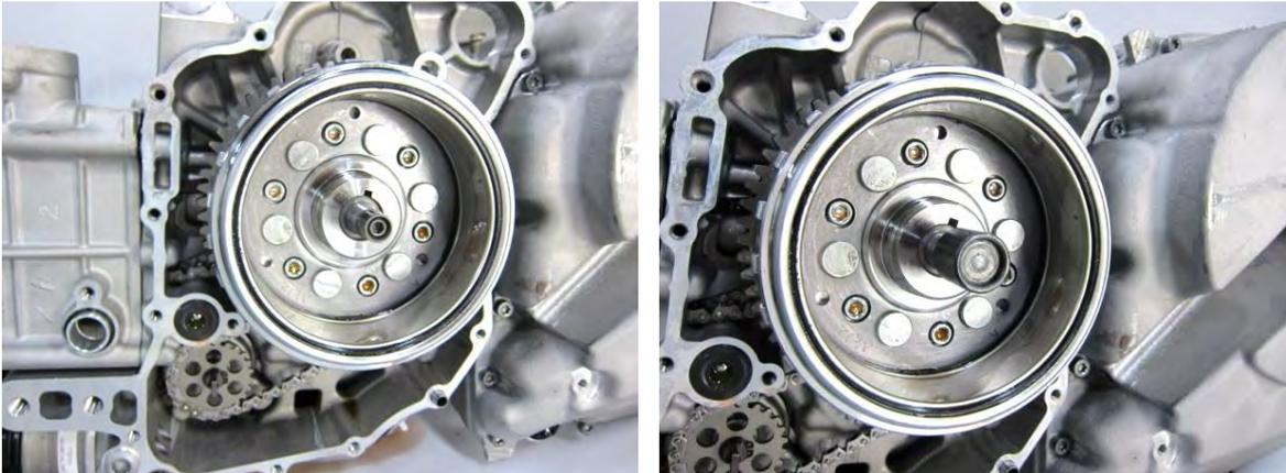
Use the special tool and remove the flywheel.
