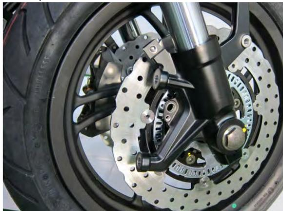
Remove the bolt of front axle.
