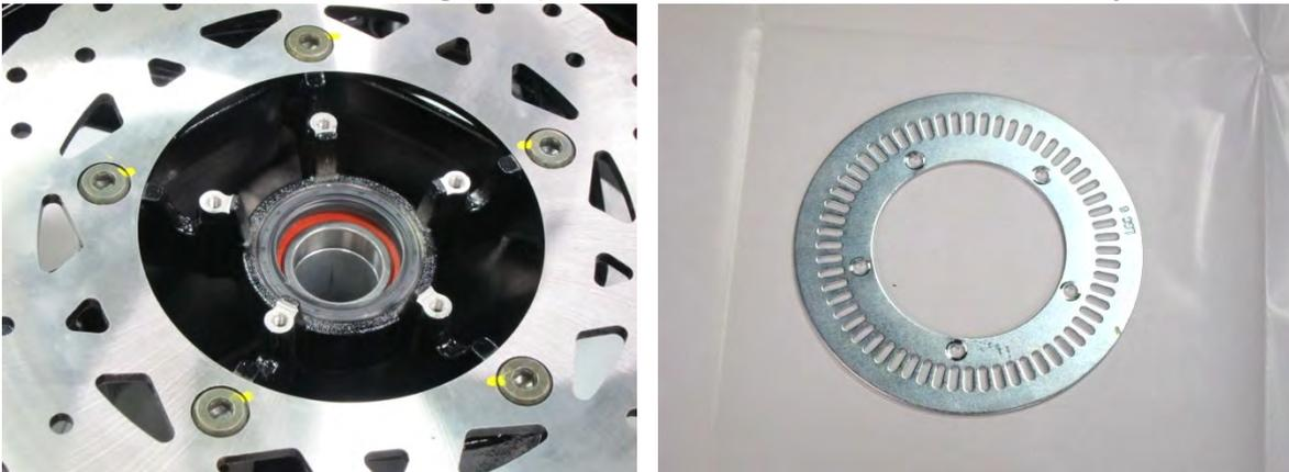
Remove the 5 bolts of the rear brake disk.
