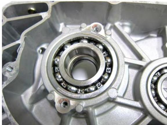
Remove the bearing by bearing puller tool.
