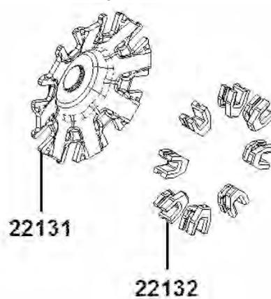
There are eight weight rollers in the back of the movable face of the drive pulley.
