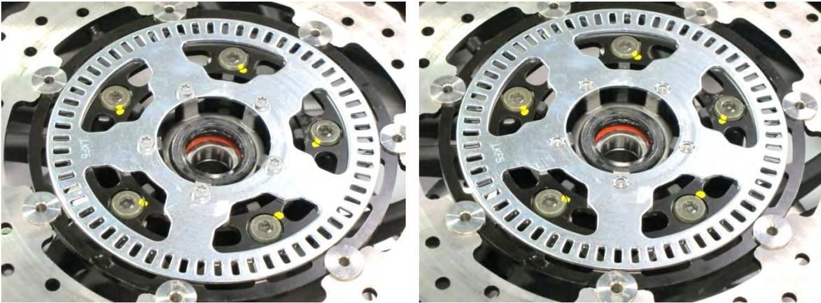
Remove the bolts of brake disk.
