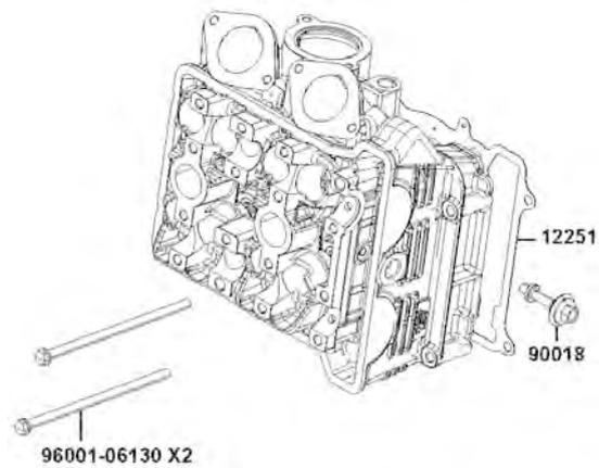
Loosen and remove the cylinder head bolts in a crisscross pattern in several steps, then remove the cylinder head.
