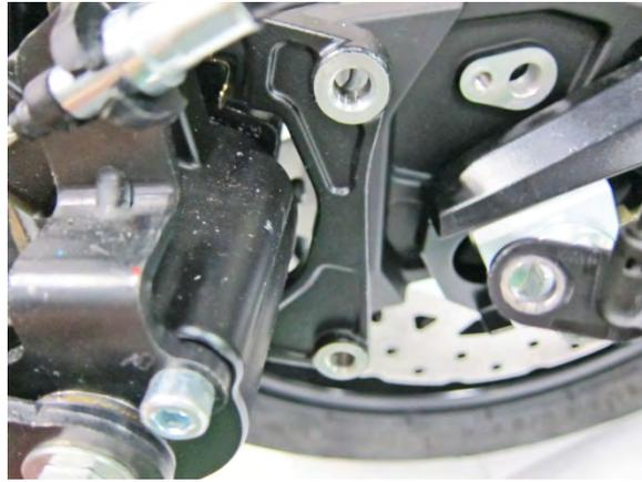
Remove the hex bolt, and separate the caliper.
