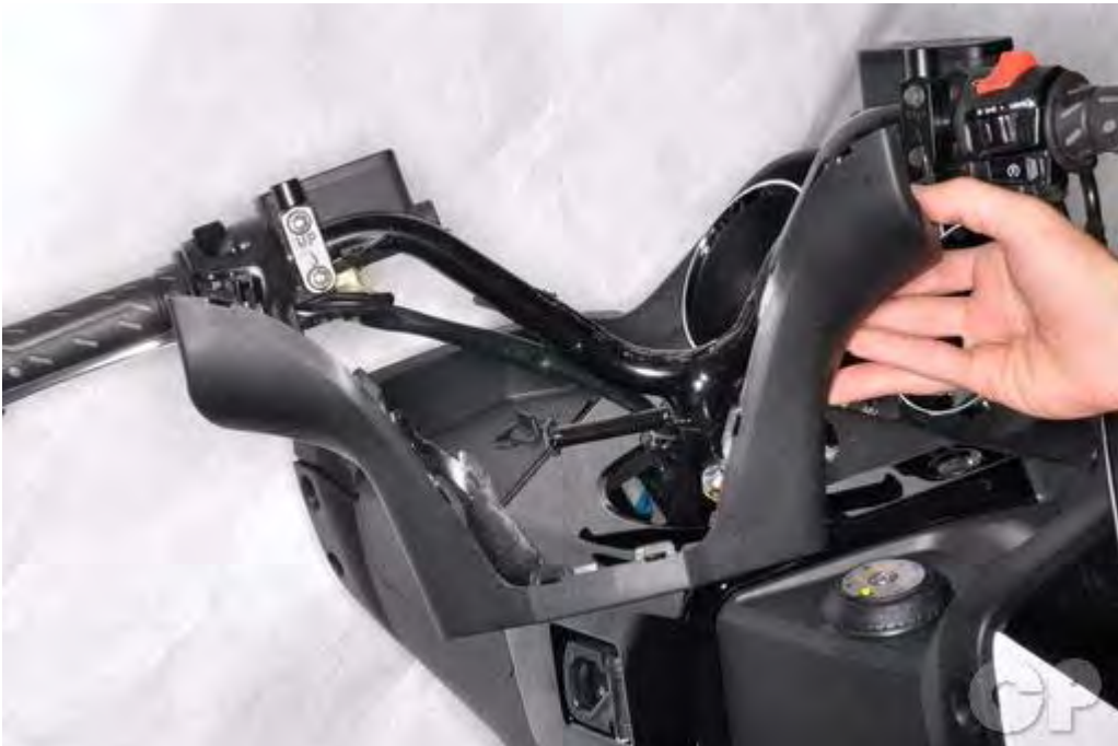
Place the lower cover onto the handlebar.
