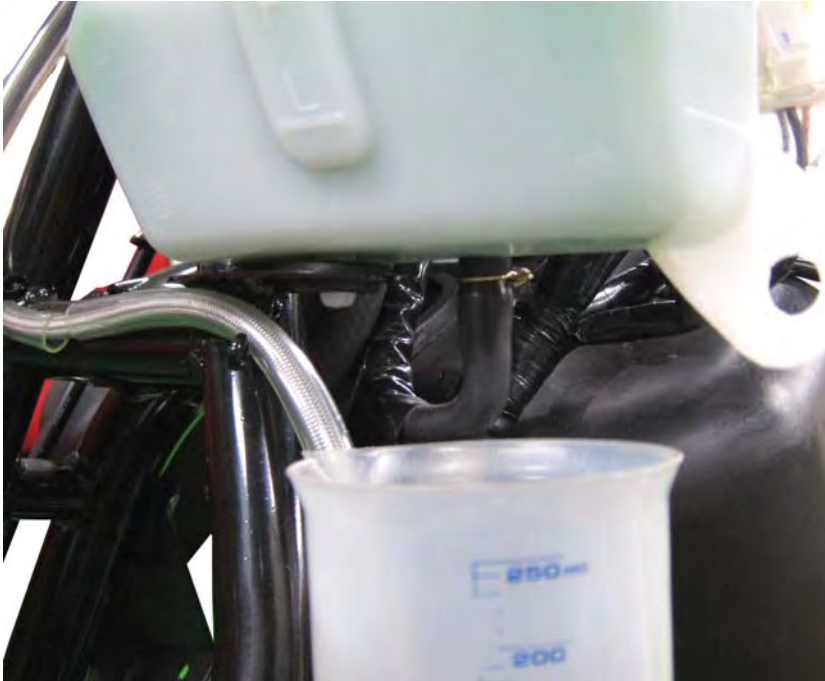
Position a suitable container below the reserve tank.
