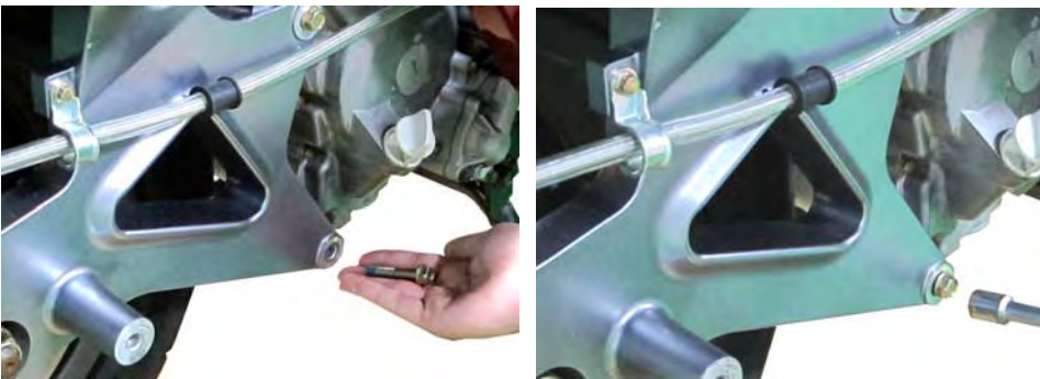
Install the two rear fork mounting bolts and tighten them securely with a 14 mm socket.
