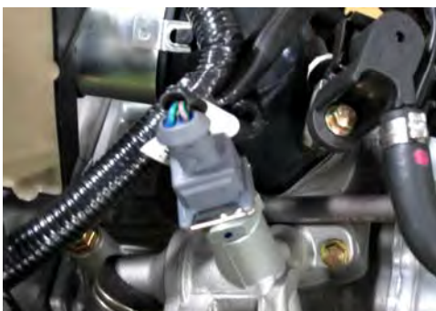
Plug in the water temperature sensor connector.
