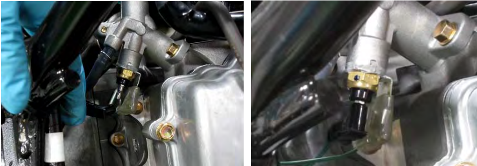
Plug in the thermostensor unit and ground connectors.
