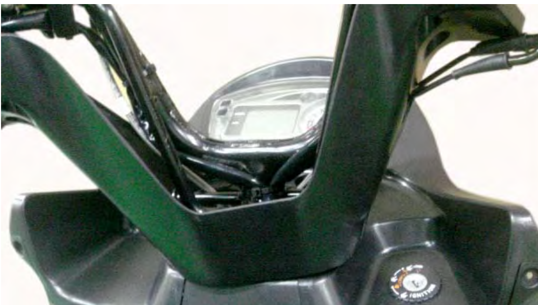
Place the lower cover onto the handlebar.
