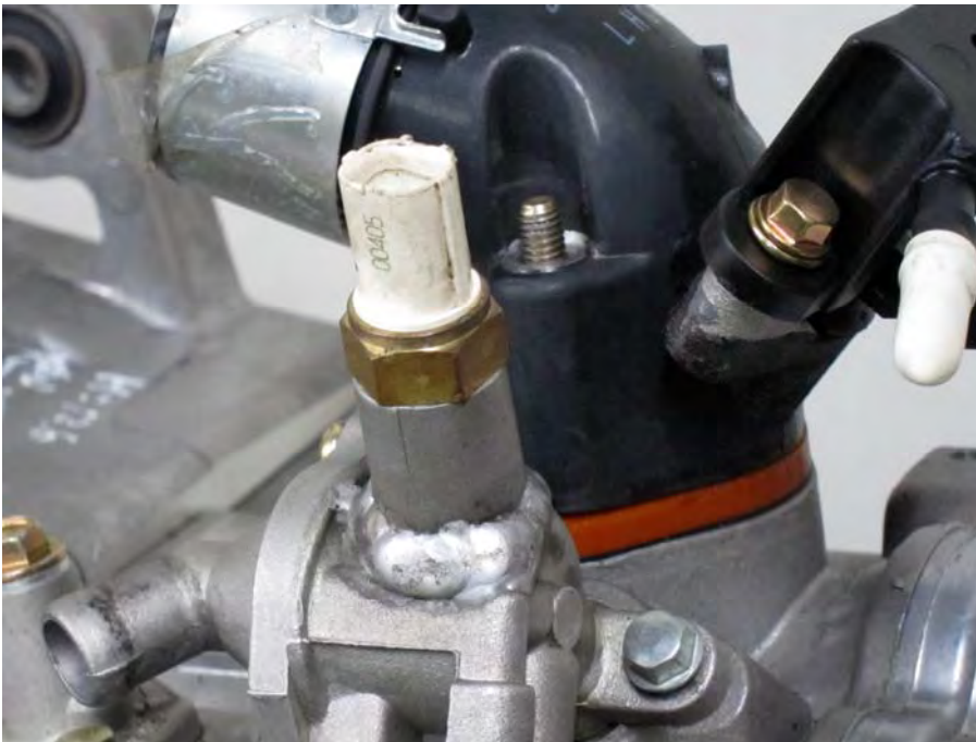
Install the WTS with a new O-ring. Tighten the WTS to specification with a 17 mm wrench.
