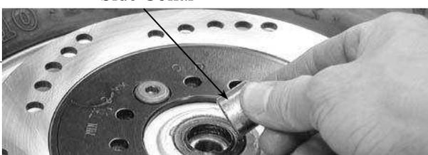
Apply grease to a new dust seal lip and
