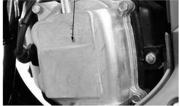
Remove the cam chain tensioner cap screw and the O-ring.
