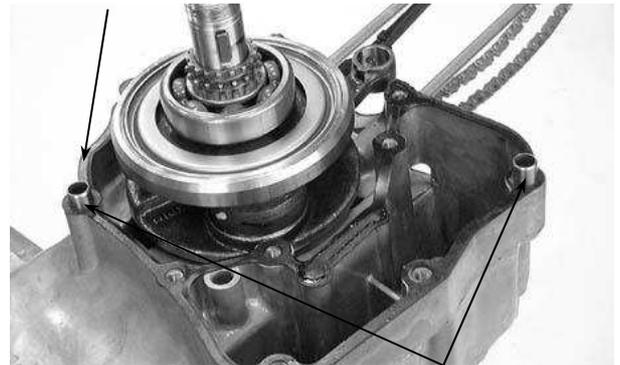
Remove the crankshaft and cam chain from the left crankcase.
