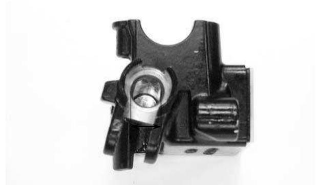
Measure the brake master cylinder piston O.D.
