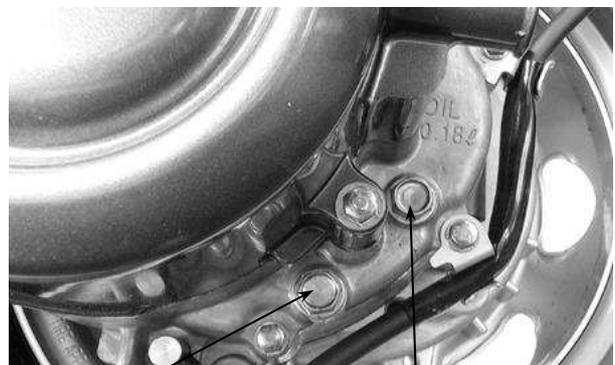
Drain Bolt Oil Check Bolt Hole/Oil Filler
