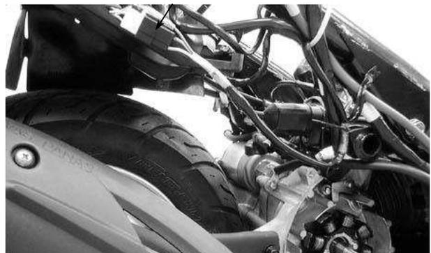
Remove the A.C. generator wire set plate.
