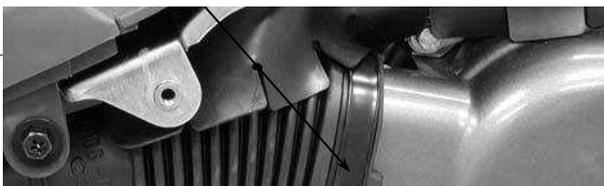
Install the drive belt air tube and tighten the
