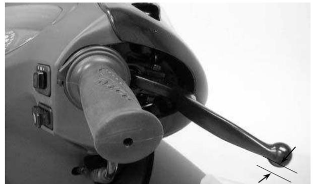
If the free play do not fall within the limit, adjust by turning the adjusting nut.
