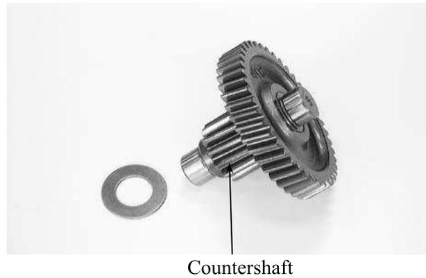
Inspect the final gear and final shaft for wear, damage or seizure.
