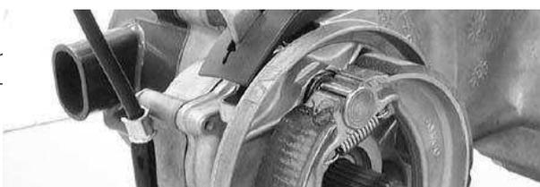
Apply engine oil to the felt seal and install it
