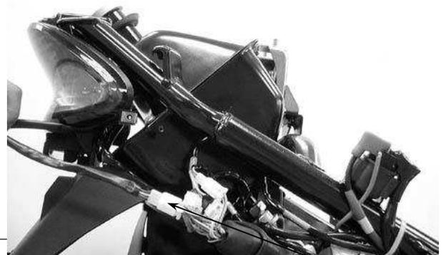
Be careful not to bend or damage the fuel unit float arm.
