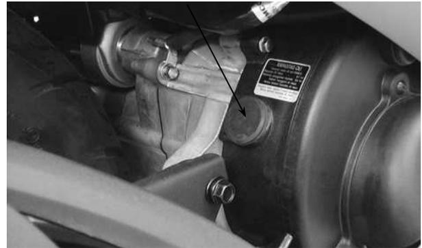
Check the ignition timing with a timing light.
