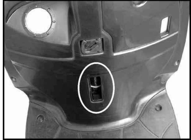
Location of Frame Serial Number
