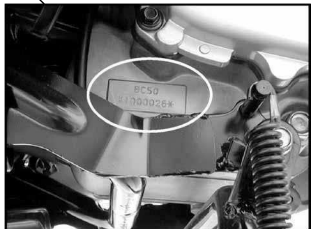
Location of Engine Serial Number
