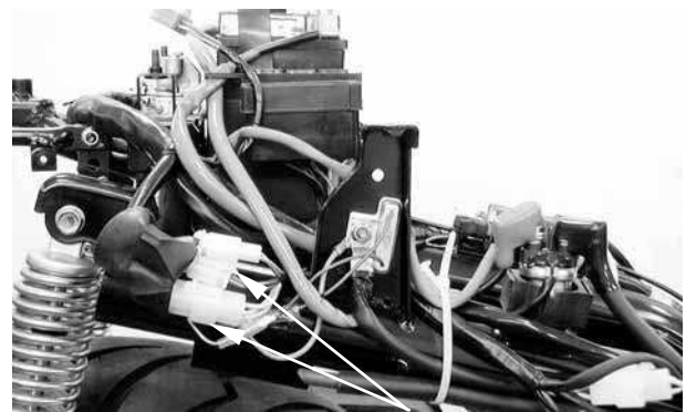
A.C. Generator Wire Connectors
