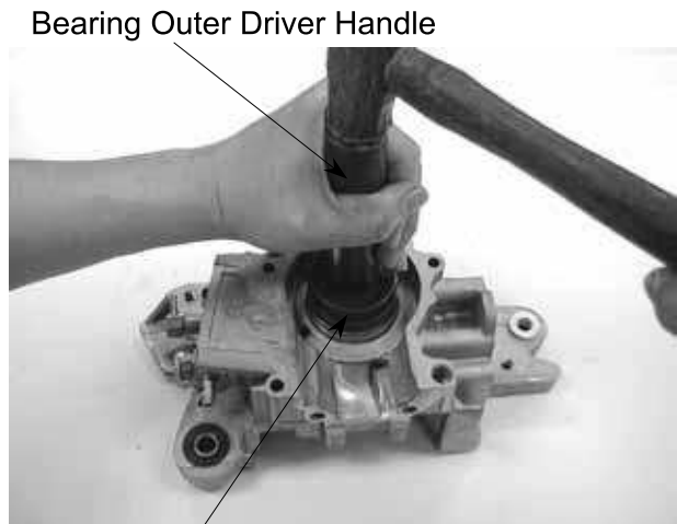
Bearing Outer Driver, 37x40mm Bearing Driver Pilot, 17mm
