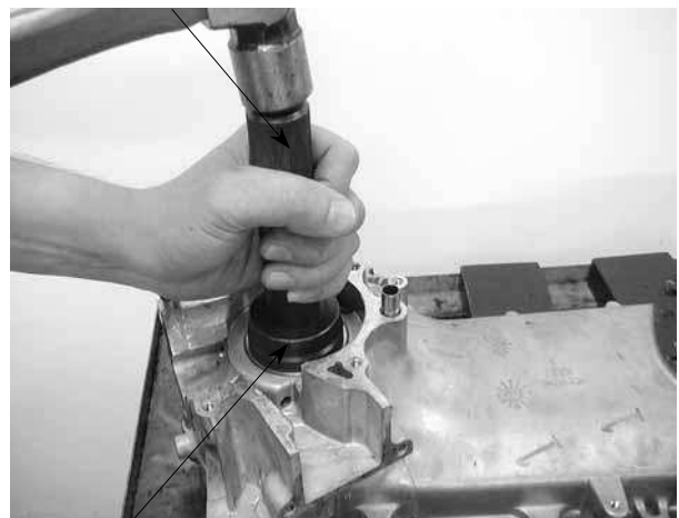
Bearing Outer Driver, 42x47mm Pilot, 20mm
