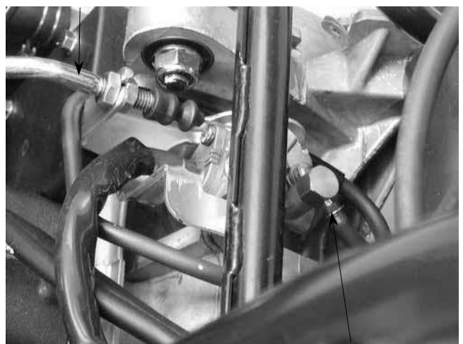
Oil Outlet Line
