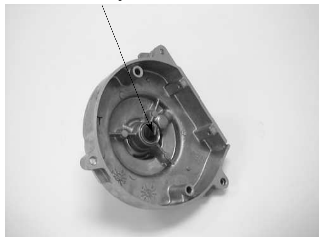
Water Pump Shaft
