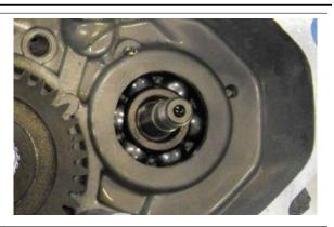
Remove the countershaft from the alternator side.
