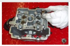
Compress the valve spring using the tool.
