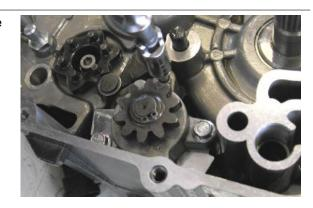
Remove the gear spider screw, unscrewing and removing the fixing screw.
