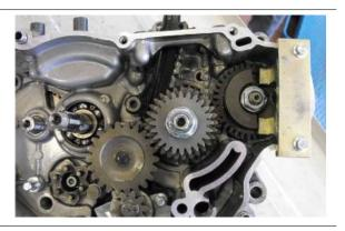
Unscrew and remove the nut and collect the washer
