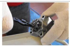
• Remove the pump gear.
