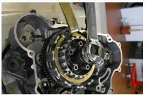
Remove the shim and the clutch housing.
