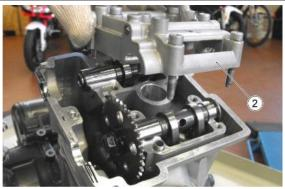
Remove the two camshafts, intake and exhaust side.
