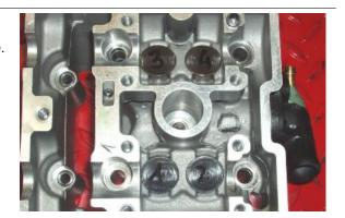
• Remove the valve bucket tappets.
