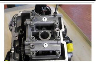
• Remove the valve cam tower (2).
