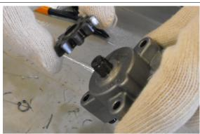
• Remove the pump gear.
