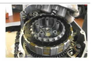
Release the screw by lowering the lock tab.
