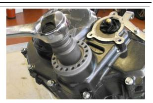
• Remove the spring and oil filter.
