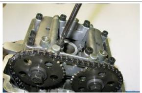
Remove the timing chain and the gears of the camshaft of the valves in question.
