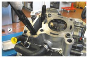
Remove the water sleeve clamp (3).
