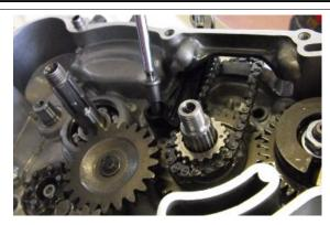
Insert the camshafts in their seats on the head, remember to position the camshaft marked with the letter (A) on the intake side and the camshaft marked with the letter (S) on the exhaust side.
