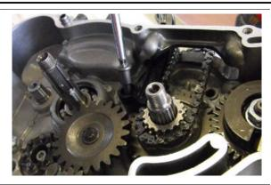
Remove the pump drive gear, removing the seeger and recovering the washer.
